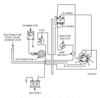
Figure 6-61.—Distributor dual lead test.
