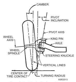
Figure 2-13.—Pivot inclination and camber.
