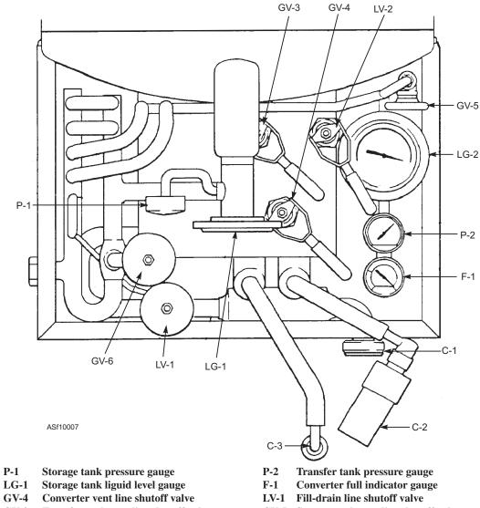
GV-4 GV-3 Transfer tank vent line shutoff valve **CV-5** Storage tank vent line shutoff valve Transfer tank fil line shutoff valve LV-2 C-2 Filler valve GV-5 Transfer tank pressure buildup valve C-3 Converter vent line connecter LG-2 Transfer tank liquid level gauge C-1 Fill-drain line coupling
