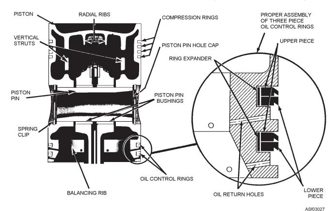
Figure 3-27.—Piston assembly of General Motors series 71 diesel engine.
