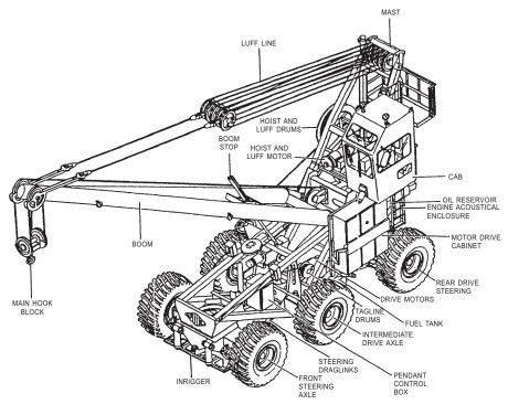
Figure 13-1.—A/S32A-36A amphibious assault crash crane (AACC).
