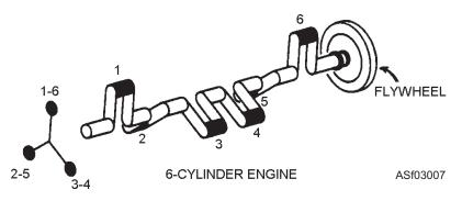
Figure 3-7.—Crankshaft for a 6-cylinder engine.
