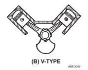
Figure 3-9.—Typical cylinder arrangements.
