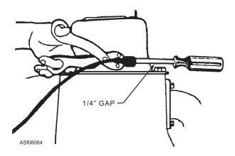
Figure 6-64.—Checking for spark at the plug.
