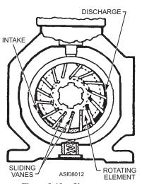
Figure 8-12.—Vane pump.
