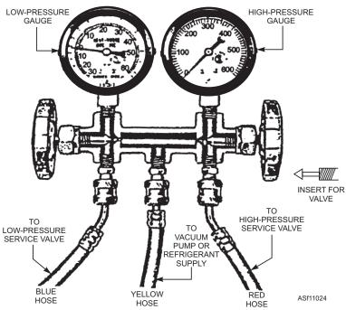
Figure 11-24.—Internal view of refrigerant manifold test set.
