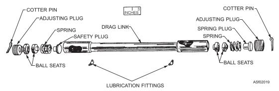
Figure 2-19.—Drag link assembly—exploded view.
