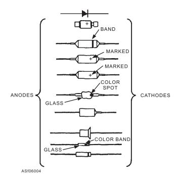
Figure 7-4.—PN diode identification.
