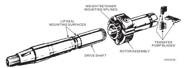
Figure 4-38.—Pump rotating parts (Model DC).
