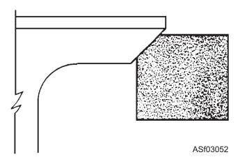
Figure 3-52.—Normal valve seat.
