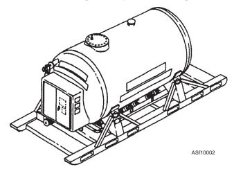
Figure 10-2.—2,000 gallon capacity liquid oxygen storage tank.
