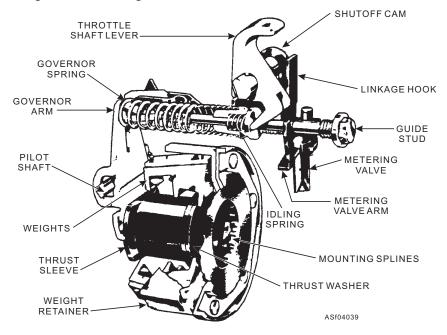
Figure 4-39.—Governor assembly (Model DC).
