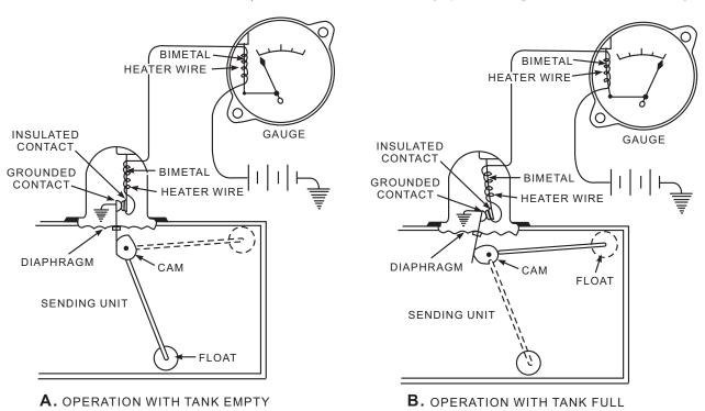
Figure 6-76.—Thermostatic fuel gauge circuit.
