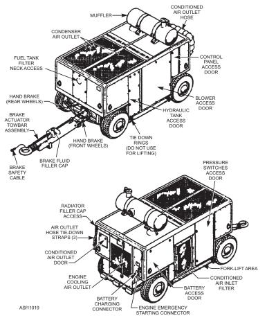
Figure 11-19.—A/M32C-17 trailer-mounted air-conditioning unit, diesel-powered.
