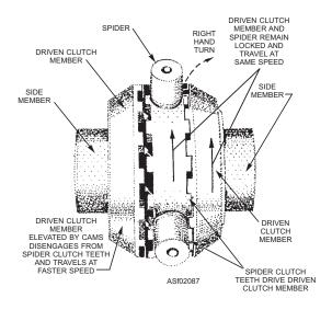
Figure 2-87.—Operation of no-spin differential during a turn.
