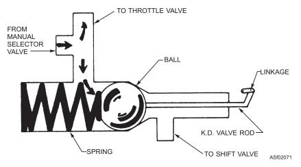
Figure 2-71.—Kickdown valve (separate valve arrangement).
