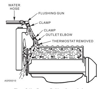
Figure 5-10.—Reverse flushing of water jackets.
