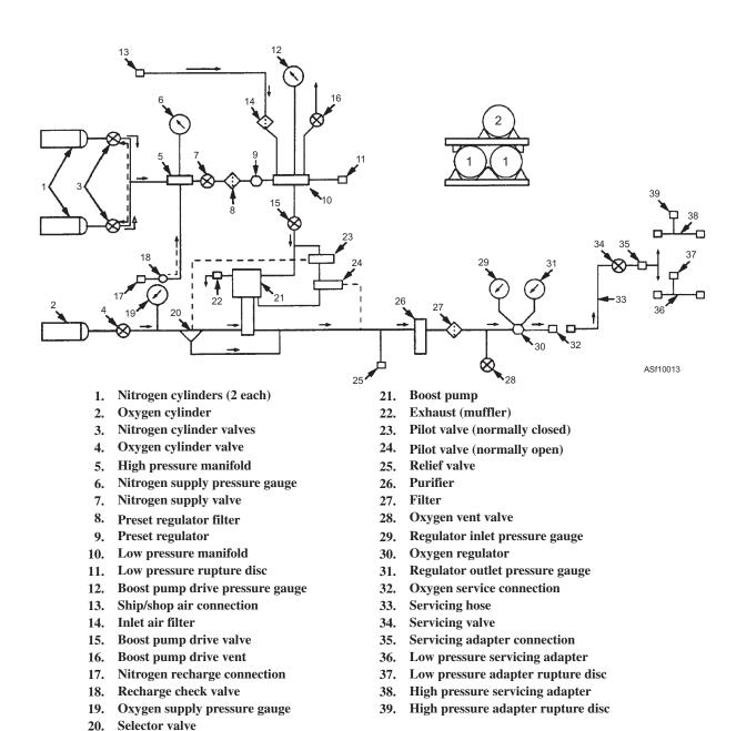
Figure 10-13.—Air/nitrogen boost pump drive and oxygen servicing flow schematic.
