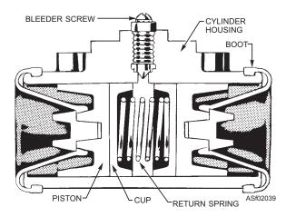
Figure 2-39.—Hydraulic brake wheel cylinder.
