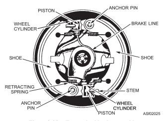
Figure 2-25.—Front wheel brake assembly.
