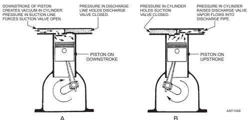
Figure 11-6.—Operating cycle of a reciprocating compressor.
