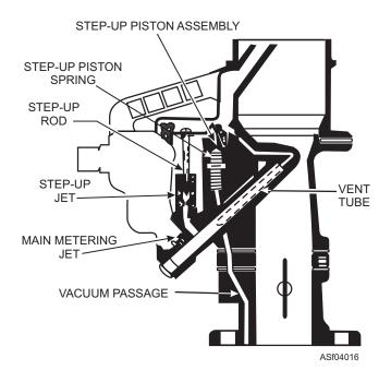
Figure 4-16.—Vacuum set-up high-speed circuit.
