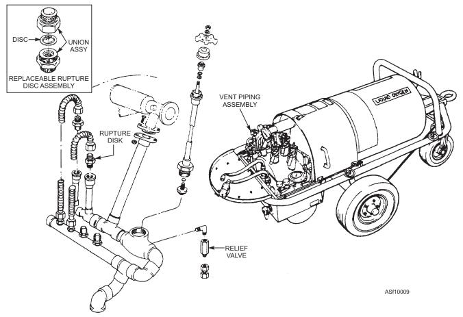
Figure 10-9.—Relief valve and rupture disc.
