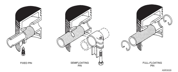
Figure 3-29.—Piston pin types.
