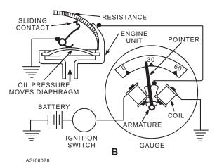
Figure 6-78.—(A) Oil pressure sending unit; (B) Schematic diagram of balancing coil oil pressure indicating system.
