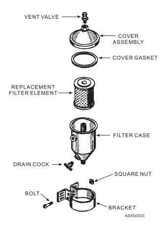
Figure 4-33.—Fuel filter assembly with replaceable element.
