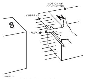
Figure 6-13.—Left-hand rule for generators.
