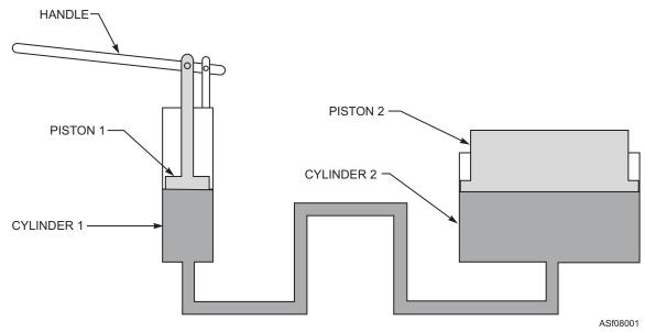
Figure 8-1.—Transmission of force by liquids.
