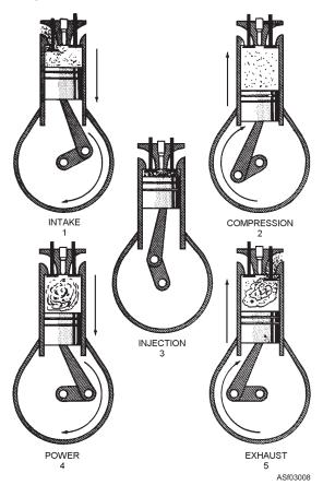
Figure 3-8.—Four-stroke cycle diesel engine.
