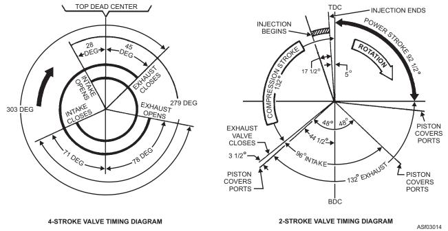
Figure 3-14.—Typical valve timing diagrams.
