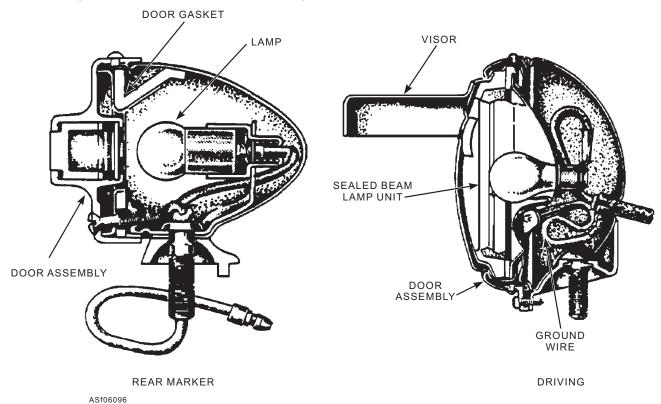
Figure 6-96.—Rear marker and blackout driving lights.
