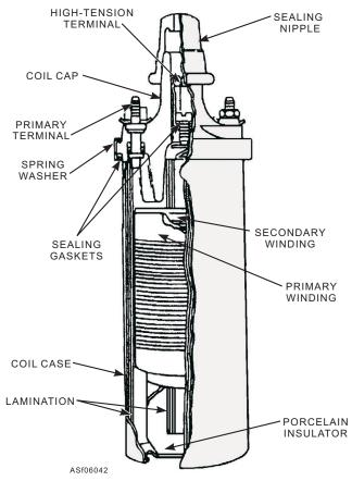
Figure 6-42.—Cutaway view of an ignition coil.
