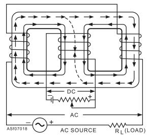
Figure 7-18.—Magnetic amplifier with three-legged core.
