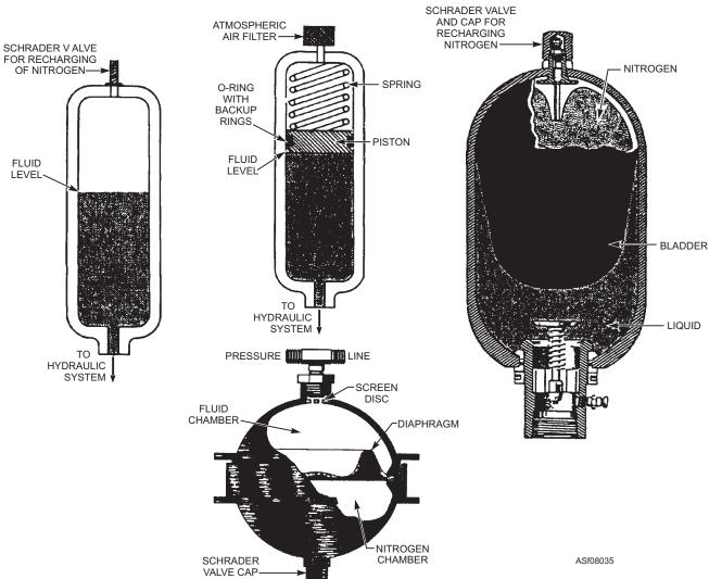
Figure 8-35.—Typical accumulators.
