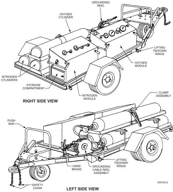
Figure 10-12.—A/U26U-1 oxygen servicing unit.
