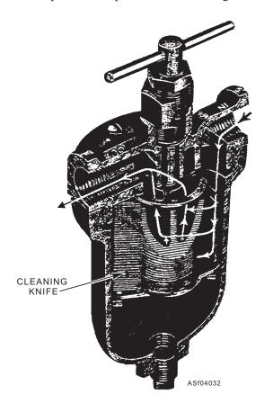
Figure 4-32.—Metal disc fuel filter.
