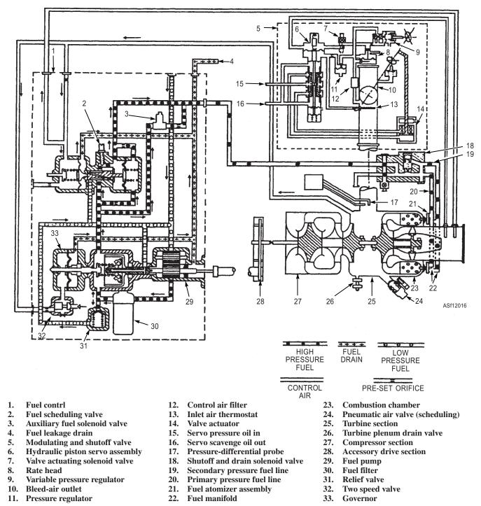
Figure 12-16.—Engine fuel and control air system and bleed-air system schematic for typical GTCP-100.
