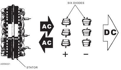
Figure 6-21.—Function of the alternator diode.
