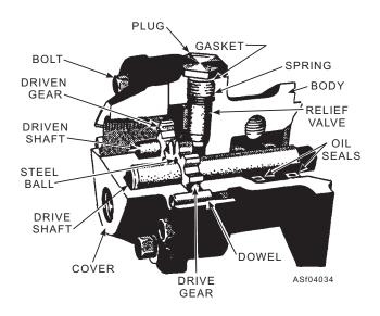
Figure 4-34.—Typical gear fuel pump assembly.
