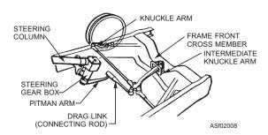
Figure 2-8.—Steering assembly.
