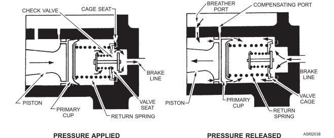
Figure 2-38.—Hydraulic brake master cylinder—operation of two-way valve.
