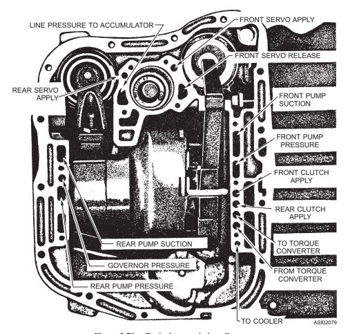
Figure 2-79.—Typical transmission oil passages.
