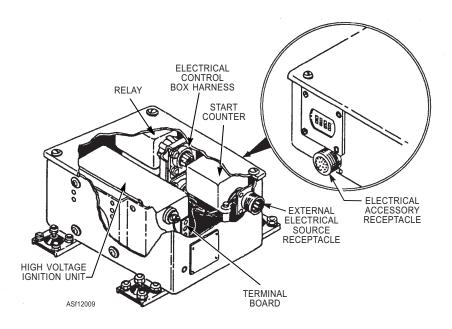
Figure 12-9.—Electrical control box.
