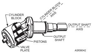
Figure 8-42.—Piston-type motor.
