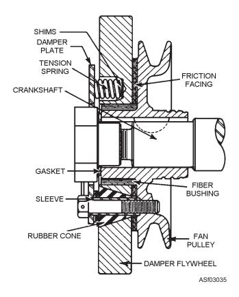
Figure 3-35.—Sectional view of a typical vibration damper.
