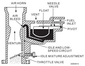
Figure 4-13.—A simple idle and low-speed circuit.
