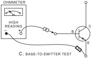
NOTE: REVERSING THE METER LEADS GIVES A LOW READING ASf07012
