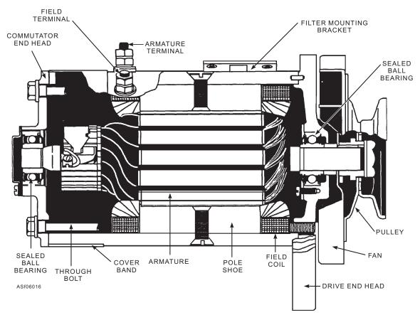
Figure 6-16.—Sectional view of dc generator.
