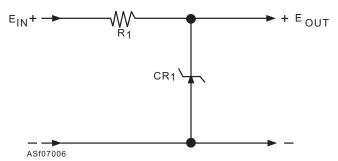
Figure 7-6.—Zener diode voltage regulating circuit.
