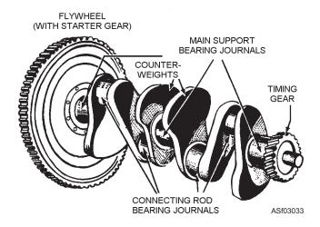
Figure 3-33.—Crankshaft of a 4-cylinder engine.
