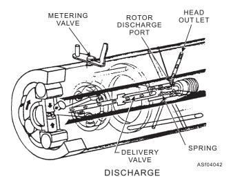
Figure 4-42.—Rotor in discharge position (DC pump).
