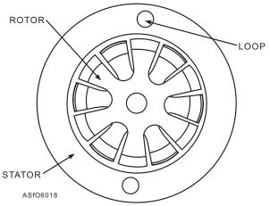
Figure 6-18.—A basic alternator with six pairs of poles in the
