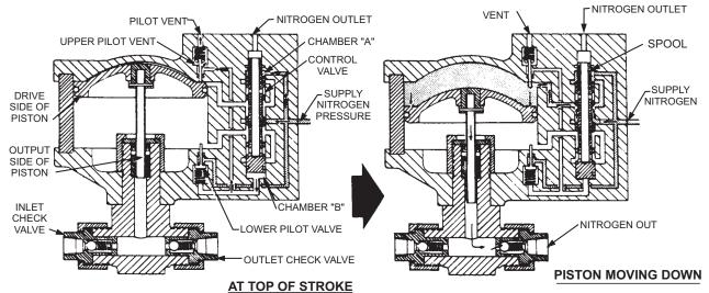
With piston in upper position, upper pilot valve is open. This exhausts chamber B. Supply nitrogen pressure in chamber A then moves control valve to DRIVE position.
