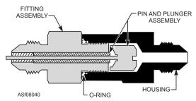
Figure 8-40.—Pressure gauge snubber.
