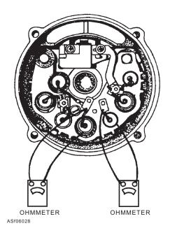
Figure 6-28.—Testing diodes with an ohmmeter.
