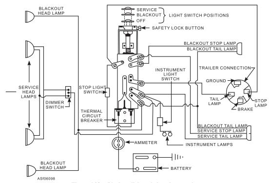
Figure 6-98.—Blackout light switch and connection.
