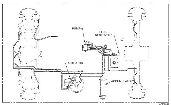
Figure 2-41.—Hydraulic system of the A/S32A-37 tow tractor.
