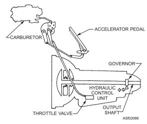
Figure 2-66.—Typical throttle valve and linkage.
