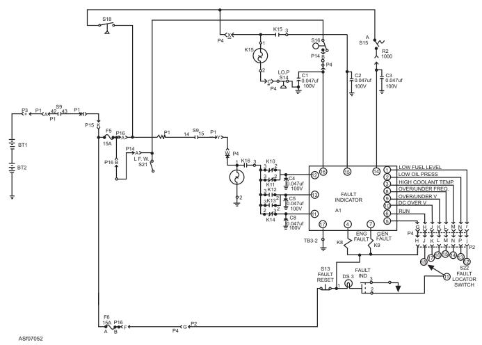
Figure 7-52.—Simplified schematic for fault locator switch.
