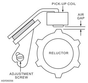
Figure 6-56.—Air gap adjustment.
