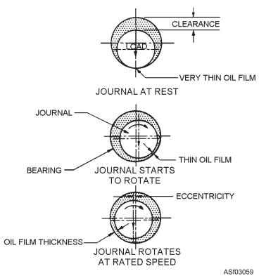
Figure 3-59.—Oil clearance between bearing and shaft.
