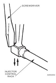
Figure 4-54.—Checking injector rack "spring" action.
