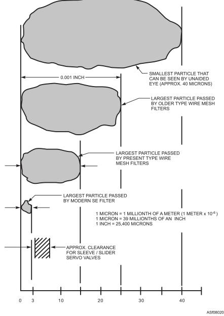
Figure 8-20.—Graphic comparison of particle sizes.
