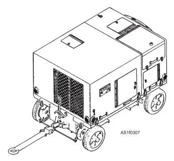
Figure 1-9.—A/M27T-7 portable hydraulic power supply.
