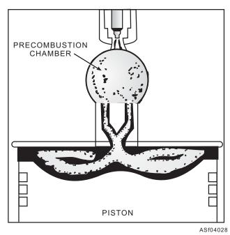
Figure 4-28.—Diesel engine precombustion chamber.
