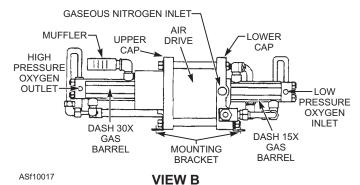
Figure 10-17.—Oxygen boost pump.
