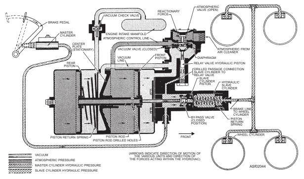
Figure 2-44.—Hydrovac operation—applied position.
