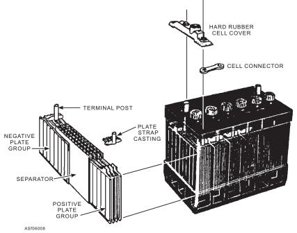
Figure 6-8.—Battery construction.
