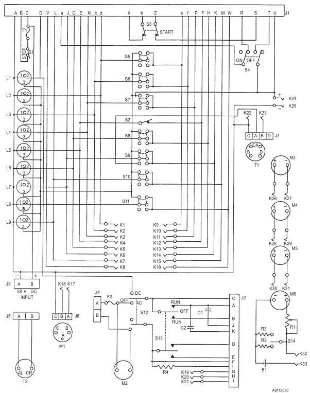
Figure 12-30.—Analyzer electrical schematic.
