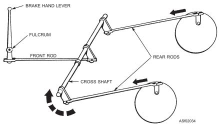
Figure 2-34.—Mechanical brake system—rods and shaft.
