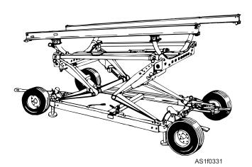
Figure 1-33.—4000A engine removal trailer.
