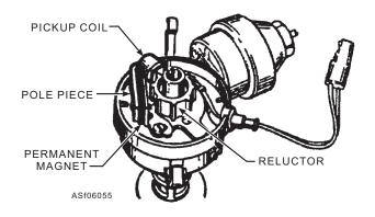
Figure 6-55.—Distributor used with transistorized ignition system.
