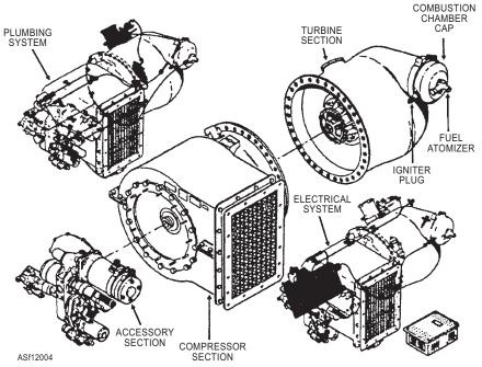
Figure 12-4.—Major sections of a gas turbine compressor (GTC-85).
