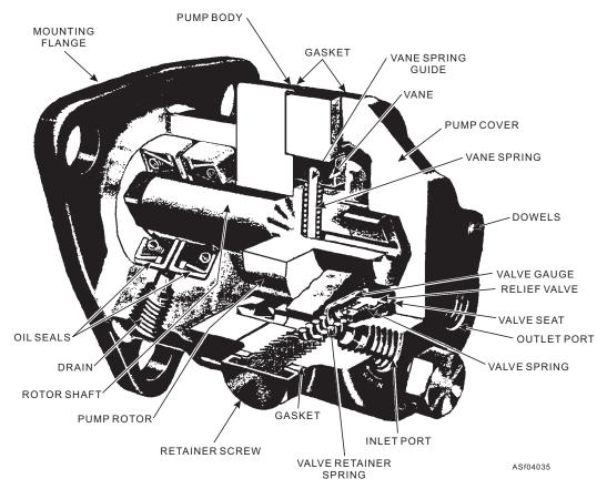
Figure 4-35.—Cutaway view of vane-type fuel pump.
