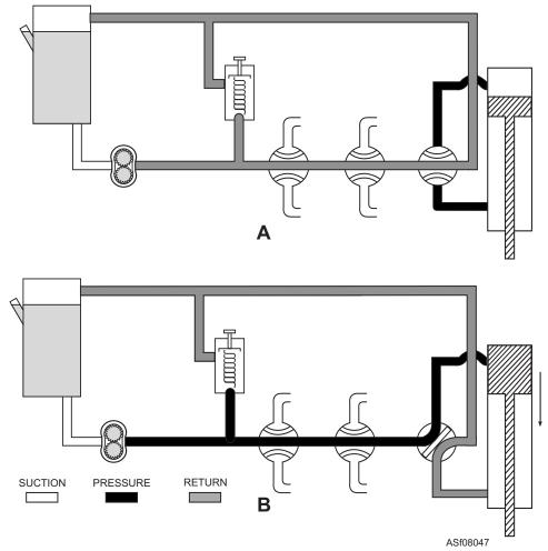
Figure 8-47.—Basic open-center system.
