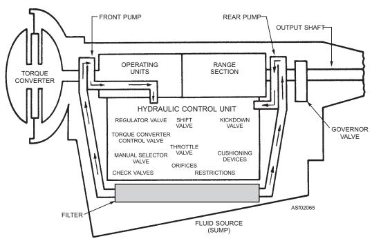
Figure 2-65.—Typical hydraulic control unit and it's components.
