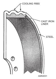
Figure 2-31.—Sectional view of a brake drum.
