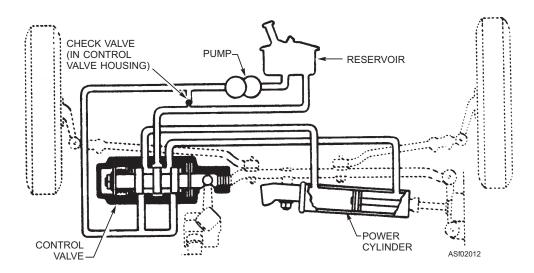
Figure 2-12.—Power steering system.
