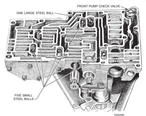
Figure 2-80.—Typical hydraulic control unit.
