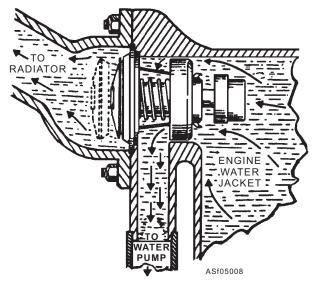
Figure 5-8.—Pellet thermostat.
