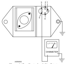
Figure 6-63.—Control unit No. 5 test.
