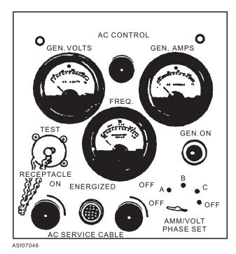
Figure 7-46.—AC Control panel.
