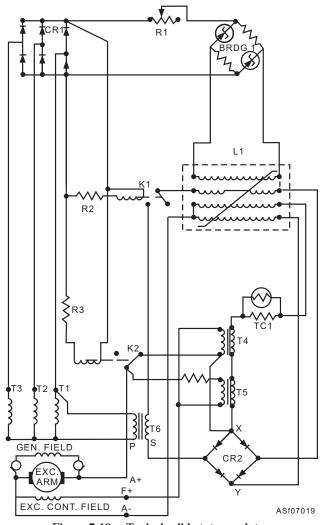
Figure 7-19.—Typical solid-state regulator.
