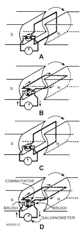
Figure 6-12.—Generating direct-current electrical energy.
