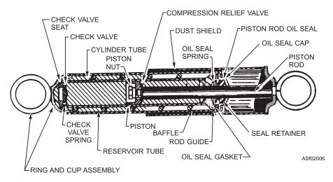
Figure 2-6.—Double-acting shock absorbers.
