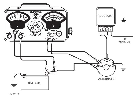
Figure 6-40.—Voltage regulator test.
