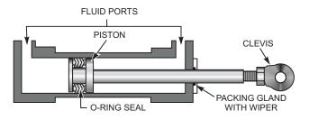
**B.** DOUBLE-ACTING PISTON ACTUATING CYLINDER AS 608037
