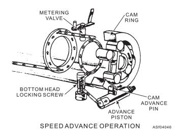
Figure 4-46.—Fuel flow in speed advance operation.
