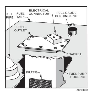
Figure 4-7.—Tank unit type of electric pump.
