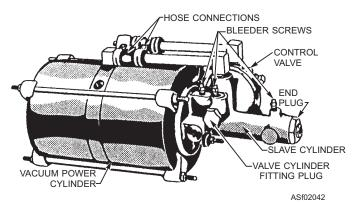
Figure 2-42.—Hydrovac vacuum power brake cylinder.
