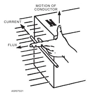
Figure 7-21.—Left-hand rule for generators.
