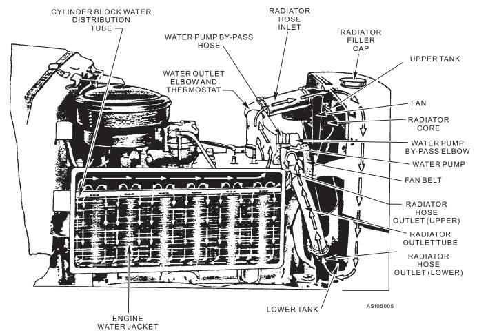
Figure 5-2.—Liquid-cooling system.
