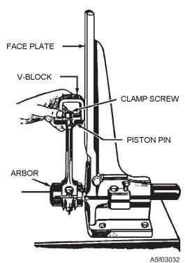
Figure 3-32.—Checking connecting rod alignment.
