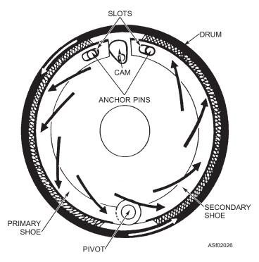
Figure 2-26.—Primary and secondary brake shoes—self-energizing action.
