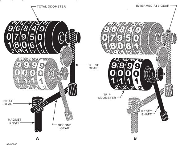
Figure 6-85.—(A) Total odometer; (B) Trip odometer.
