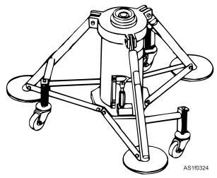
Figure 1-26.—Fixed height tripod jack.
