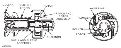
Figure 6-68.—Solenoid shift starter and overrunning clutch drive.
