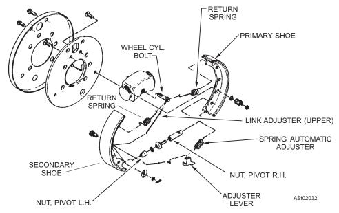
Figure 2-32.—Brake assembly, self-adjusting.
