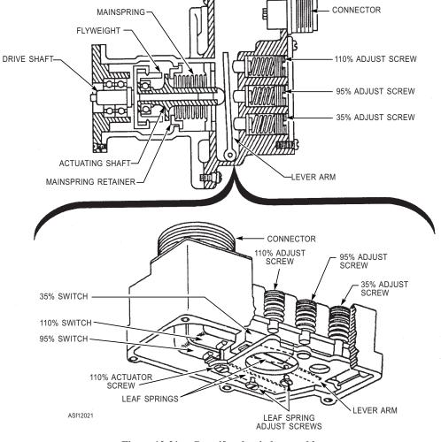
Figure 12-21.—Centrifugal switch assembly.
