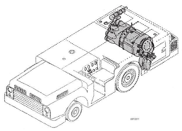
Figure 12-11.—GTCP-100 gas turbine engine in enclosure.
