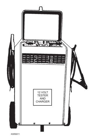
Figure 6-11.—Potable constant potential battery charger.
