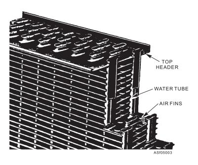
Figure 5-3.—Tubular radiator core construction.
