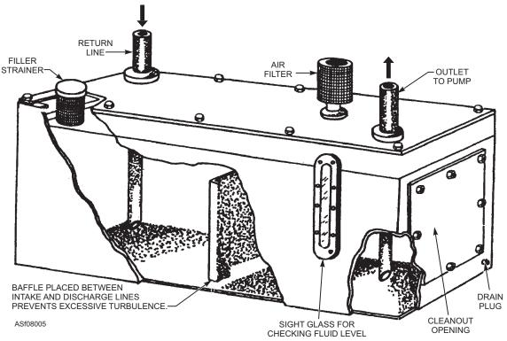
Figure 8-5.—Typical hydraulic reservoir.
