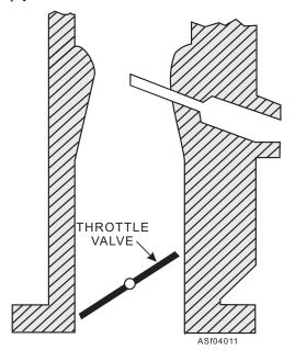
Figure 4-11.—Simplified carburetor with throttle valve.
