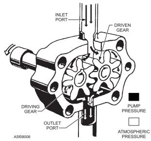
Figure 8-8.—Spur tooth pump.
