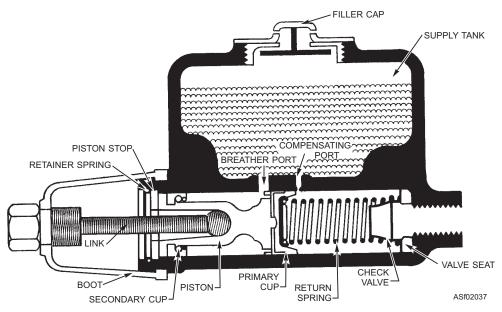
Figure 2-37.—Hydraulic brake master cylinder.
