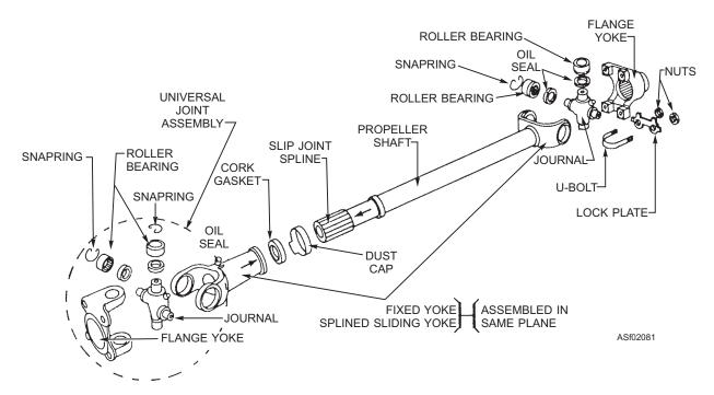
Figure 2-81.—Propeller shaft assembly.
