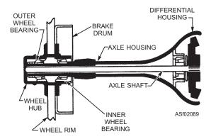
Figure 2-89.—Cross section of rear hub in full floating axle.
