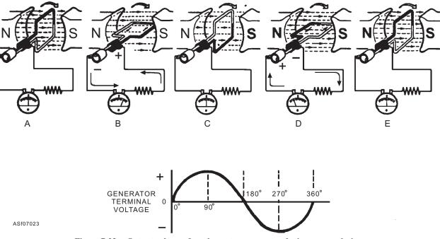
Figure 7-23.—Output voltage of an elementary generator during one revolution.
