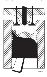
Figure 4-27.—Diesel engine open combustion chamber.
