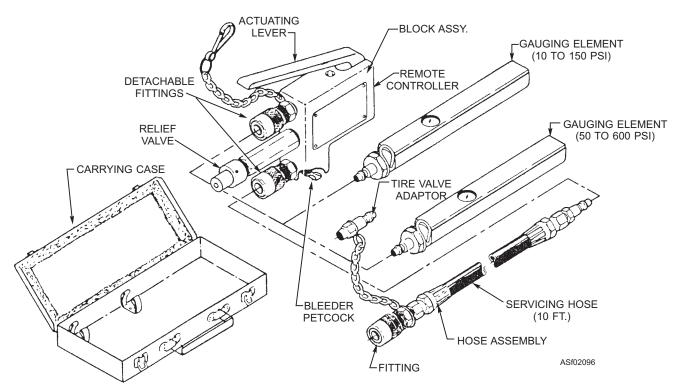
Figure 2-96.—Tire inflator assembly kit.
