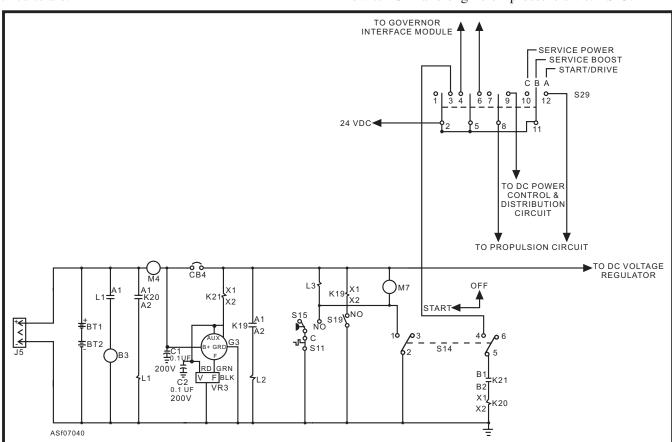
Figure 7-40.—Engine starting circuit.
