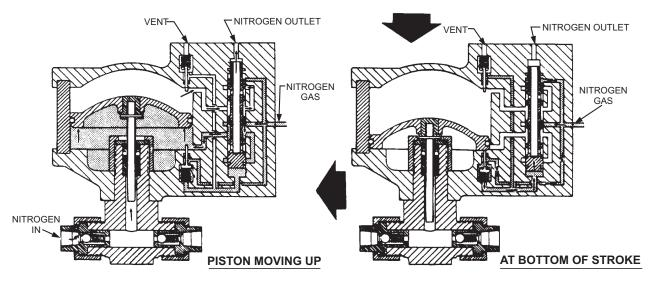
With control valve in RETURN position, supply nitrogen pressure acts on lower side of piston and moves it upward. This pushes the piston assembly up, sucking gas in thru inlet check valve. Nitrogen from upper side of piston is exhausted thru control valve spool.
