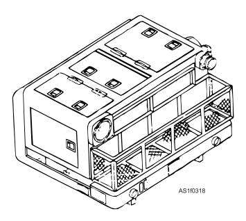
Figure 1-20.—A/S47A-1 tractor-mounted enclosure.
