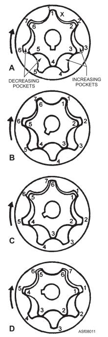
Figure 8-11.—Principles of operation of the internal gear group.
