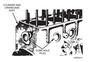
Figure 3-17.—Core hole plugs installed in cylinder block.
