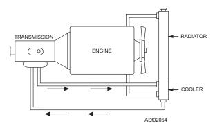
Figure 2-54.—Typical radiator-type oil cooler.
