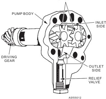
Figure 5-12.—Gear oil pump.
