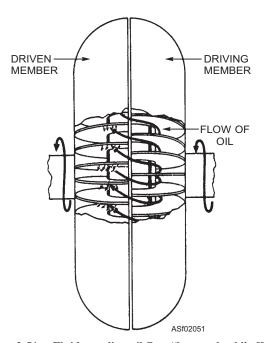
Figure 2-51.—Fluid coupling oil flow "bounce back" effect.
