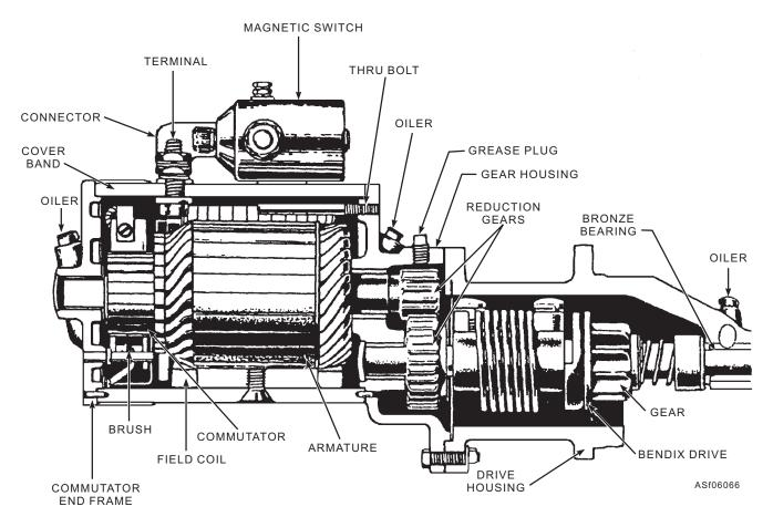
Figure 6-66.—Sectional view of a heavy-duty starter.
