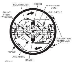
Figure 6-14.—A shunt-wound generator.
