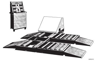
Figure 3-10.—Chassis dynamometer.
