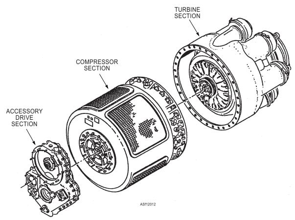
Figure 12-12.—GTCP-100 gas turbine engine sections.
