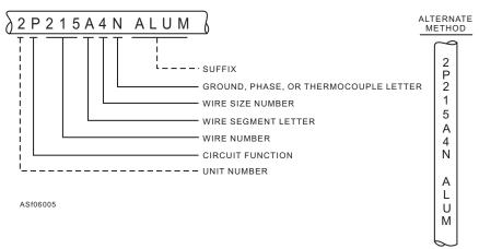
Figure 6-5.—Alphanumeric wire identification code.
