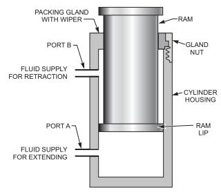
A. DOUBLE-ACTING RAM TYPE ACTUATING CYLINDER
