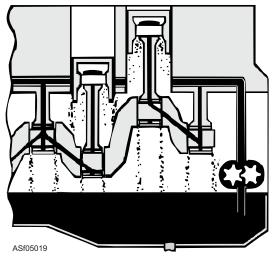
Figure 5-19.—Full force-feed lubrication system.
