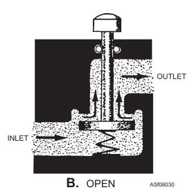
Figure 8-30.—Operation of a simple poppet valve.
