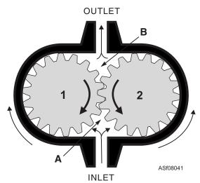
Figure 8-41.—Gear-type motor.
