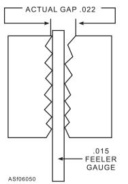
Figure 6-50.—False setting given by feeler gauge for used points.
