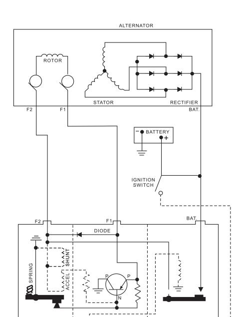
Figure 6-37.—Ac charging circuit using a semitransistorized regulator.
