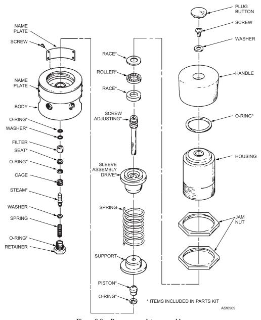
Figure 9-9.—Pressure regulator assembly.
