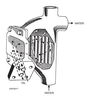
Figure 5-17.—Oil temperature regulator (cooler).
