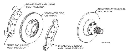
Figure 2-29.—Disc brake assembly.
