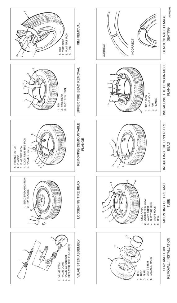
Figure 2-95.—Demountable flange teardown and buildup.
