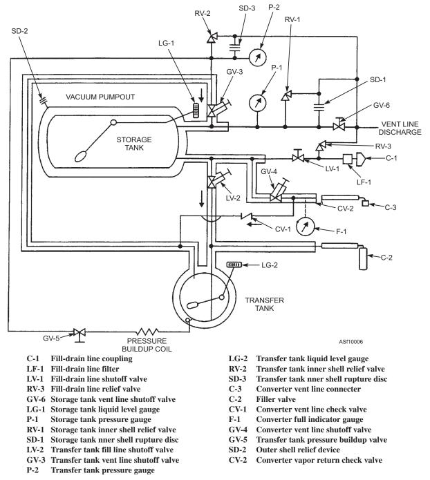
Figure 10-6.—LOX servicing trailer schematic diagram.
