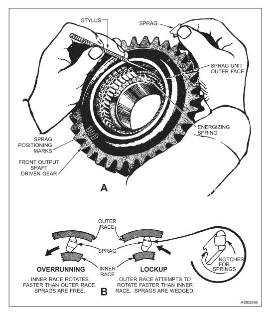
Figure 2-56.—Typical sprag assembly, overrunning clutch.
