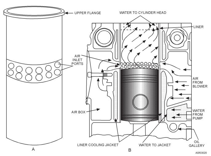
Figure 3-20.—(A) Dry-type liner for 2-cycle General Motors series engines. (B) Section through series 71 block.
