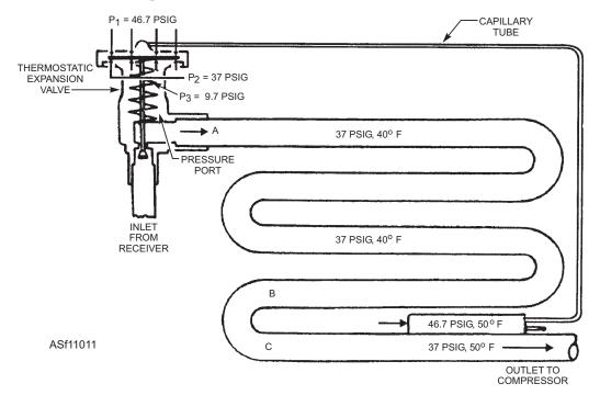
Figure 11-11.—Thermostatic expansion valve and evaporator.
