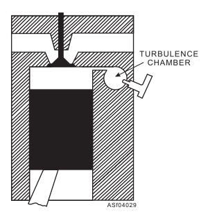
Figure 4-29.—Diesel engine turbulence combustion chamber.
