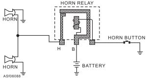
Figure 6-88.—Dual horns and relay circuit.
