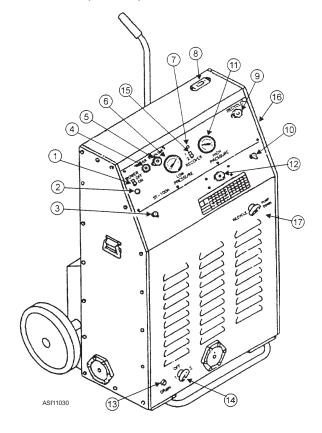
Figure 11-30.—Refrigerant recovery-recycle units.
