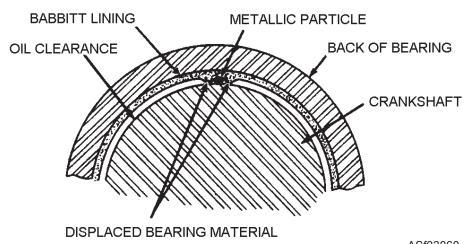
Figure 3-60.—Effect of a metallic particle embedded in bearing material (Babbit lining).
