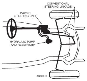
Figure 2-11.—Diagram of a power steering unit.
