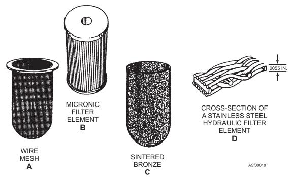
Figure 8-18.—Different types of hydraulic filter elements.
