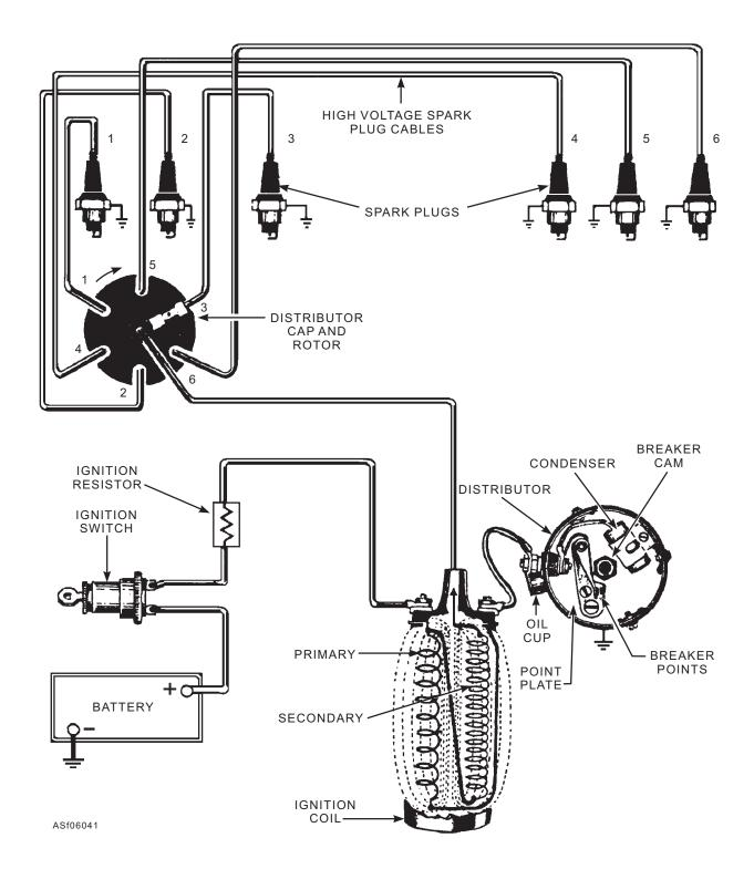
Figure 6-41.—Conventional battery ignition system.
