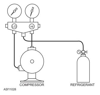
Figure 11-28.—Connections for low-side charging.
