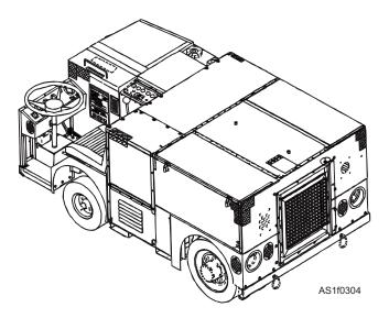
Figure 1-6.—A/S37A-3 shipboard mobile electric power plant.
