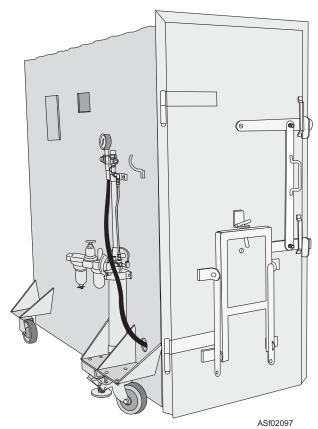
Figure 2-97.—Safety cage for inflation of tires.
