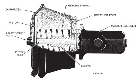
Figure 2-46.—Master cylinder assembly—air-over-hydraulic brake system.
