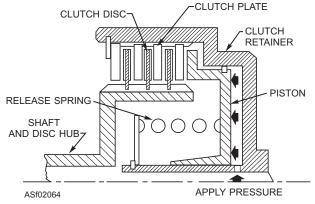
Figure 2-64.—Multiple disc clutch unit.
