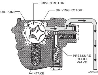
Figure 5-13.—Rotary oil pump.
