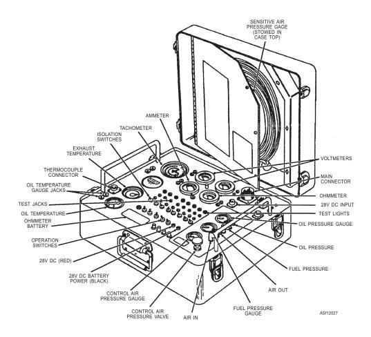
Figure 12-27.—Gas turbine engine analyzer.
