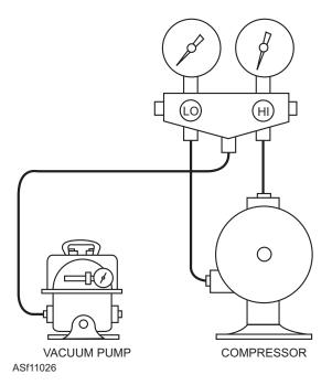
Figure 11-26.—Connections for drawing a vacuum.
