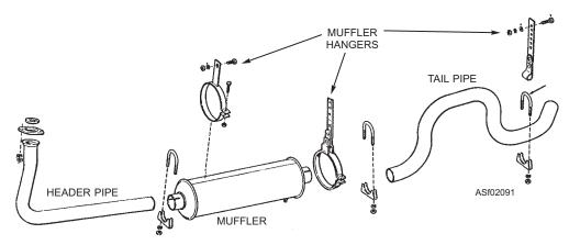
Figure 2-91.—Typical exhaust system.
