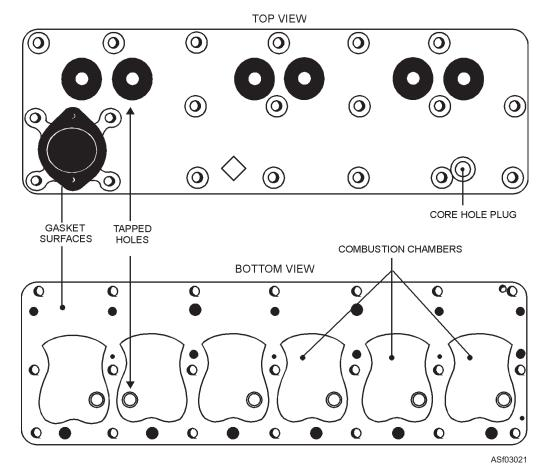
Figure 3-21.—Cylinder head for L-head engine.
