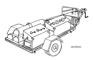
Figure 1-35.—A/U26U-1A oxygen servicing unit.
