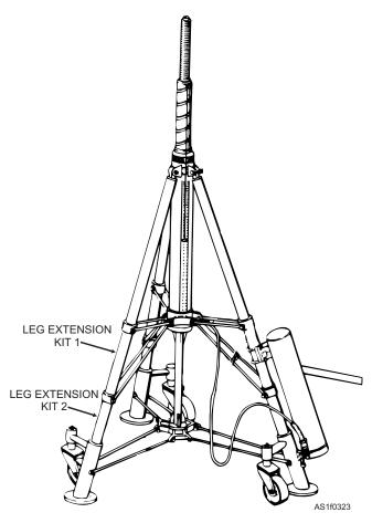
Figure 1-25.—Variable height tripod jack, two-leg extension.
