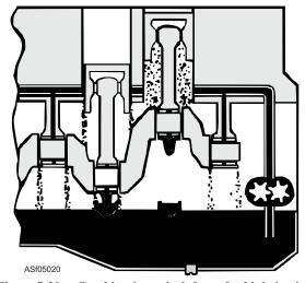
Figure 5-20.—Combination splash force-feed lubrication system.
