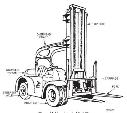
Figure 13-10.—A typical forklift.
