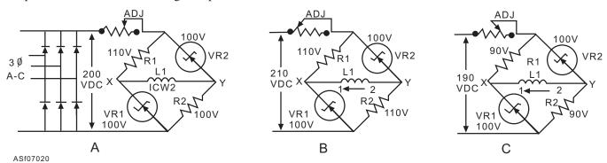
Figure 7-20.—Views of line voltage-sensing bridge (BRDG).
