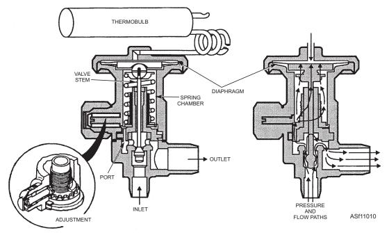
Figure 11-10.—Thermostatic expansion valve.
