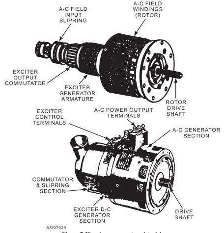
Figure 7-29.—An ac generator pictorial.
