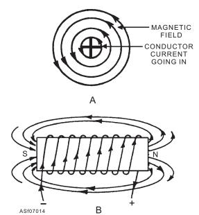
Figure 7-14.—Magnetic field of a current-carrying conductor.
