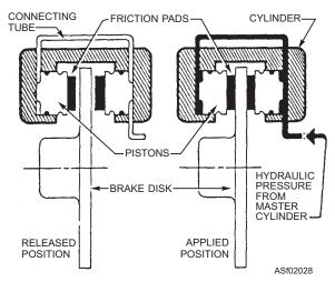
Figure 2-28.—Sectional view of a disc brake in released and applied position.
