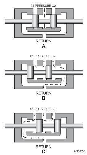
Figure 8-33.—Closed-center directional control valve.
