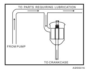
Figure 5-16.—Partial flow filter.
