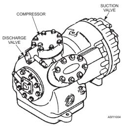
Figure 11-4.—Reciprocating semi-hermetic compressor.
