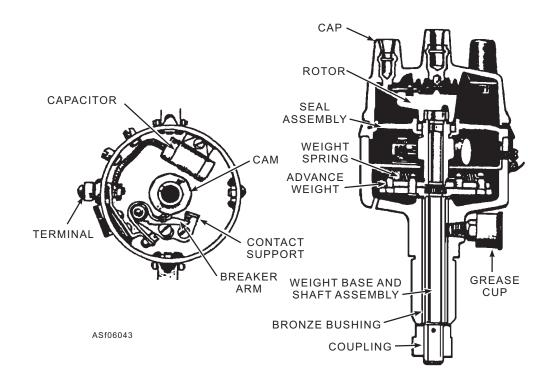
Figure 6-43.—Side and top view of a distributor.
