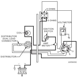
Figure 6-58.—Harness connector No. 2 test.
