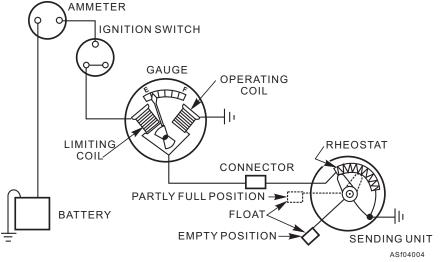
Figure 4-4.—Coil-type gauge circuit.
