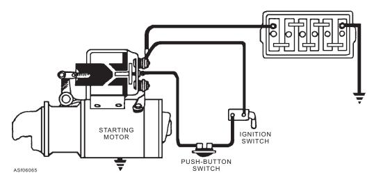
Figure 6-65.—Electric starting system.
