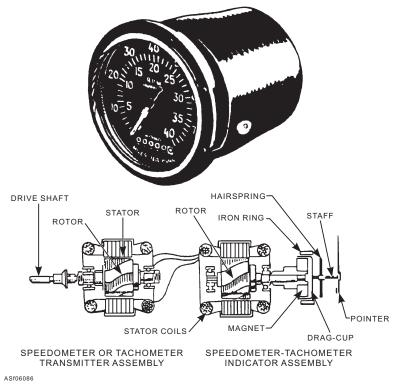
Figure 6-86.—Electrical speedometer-tachometer.
