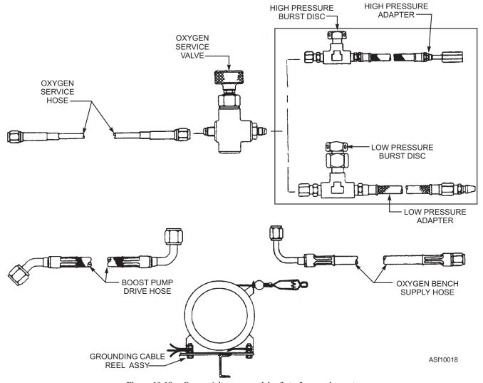
Figure 10-18.—Oxygen/nitrogen servicing/interface equipment.
