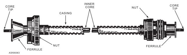
Figure 6-83.—Speedometer and tachometer drive shaft.
