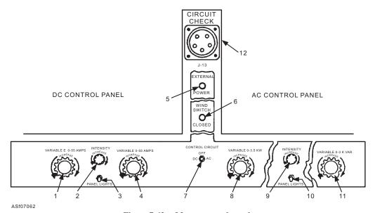
Figure 7-62.—Master control panel.
