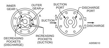
Figure 8-10.—Internal gear pump.
