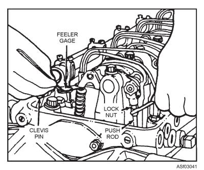
Figure 3-41.—Adjusting valve clearance.
