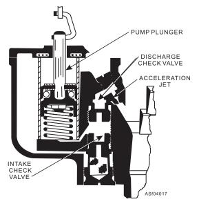
Figure 4-17.—Carburetor accelerator pump circuit.
