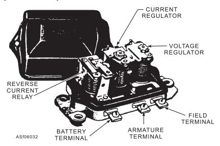
Figure 6-32.—Three-unit, vibrating contact, dc regulator.
