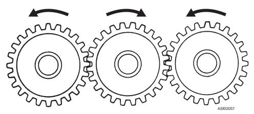
Figure 2-57.—Direction of gear rotation.
