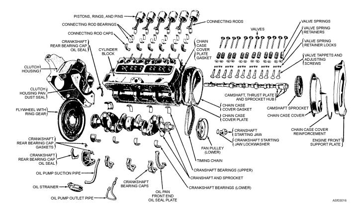
Figure 3-16.—Cylinder block and components.
