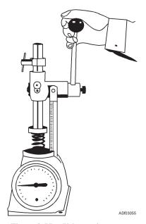
Figure 3-55.—Valve spring tester.
