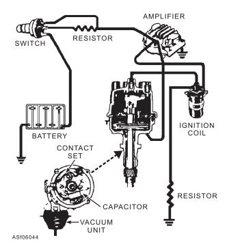
Figure 6-44.—Contact controlled transistor battery ignition system.
