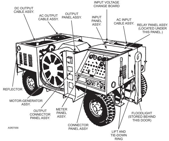
Figure 7-56.—MMG-1A mobile motor-generator set (internal view).
