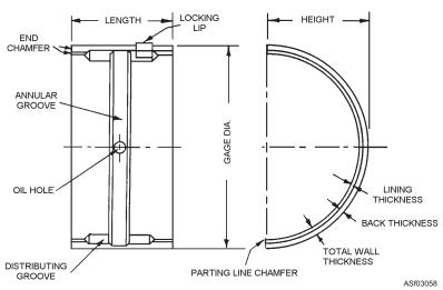
Figure 3-58.—Typical sleeve-type bearing half.
