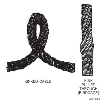
Figure 13-8.—Cable damage resulting from a pulled-through
