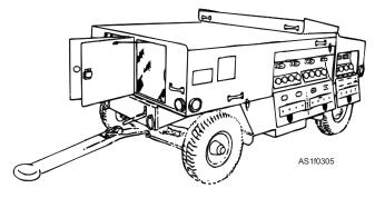
Figure 1-7.—DA-675/MSM dummy load electric unit.
