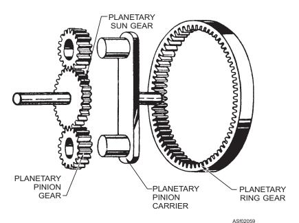
Figure 2-59.—Members of a simple planetary gear system.
