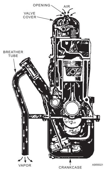
Figure 5-21.—Crankshaft breather tube.
