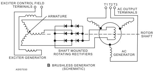
Figure 7-30.—Ac generator schematic drawings.
