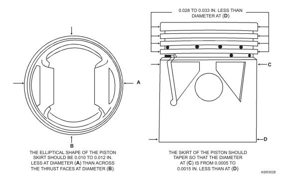
Figure 3-28.—Cam-ground piston.
