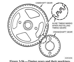
Figure 3-56.—Timing gears and their markings.
