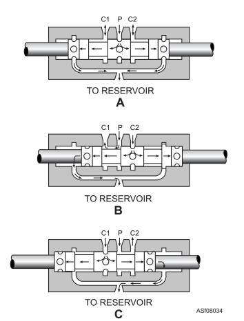
Figure 8-34.—Open-center directional control valve.
