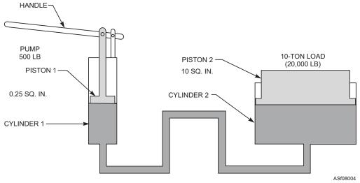
Figure 8-4.—A 10-ton hydraulic jack.
