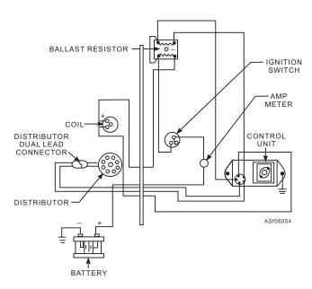
Figure 6-54.—Electronic ignition system.
