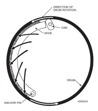
Figure 2-24.—Brake shoe self-energizing action.
