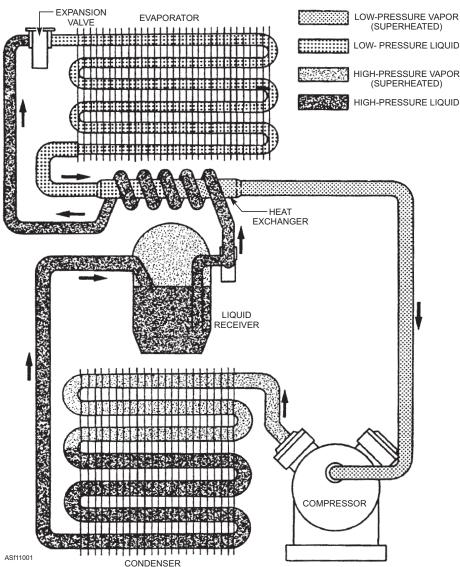
Figure 11-1.—Fundamental refrigeration cycle.
