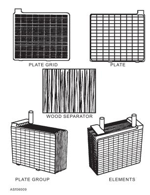
Figure 6-9.—Cell element construction.
