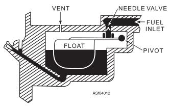
Figure 4-12.—A typical float circuit.
