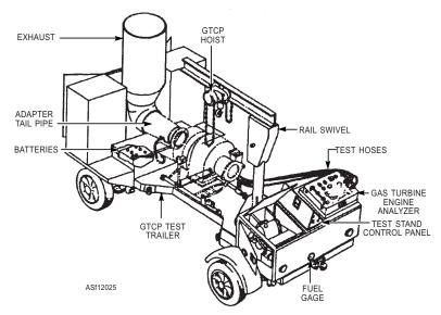
Figure 12-25.—Gas turbine engine test stand.
