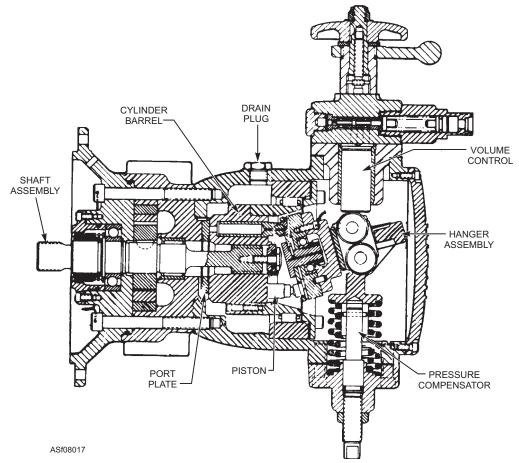
Figure 8-17.—Variable displacement axial piston pump.
