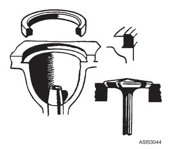
Figure 3-44.—Valve seat insert.
