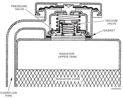
Figure 5-4.—Radiator pressure cap.
