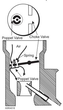
Figure 4-18.—Spring-loaded poppet valve in choke valve.
