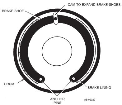
Figure 2-22.—Internal expanding brake.
