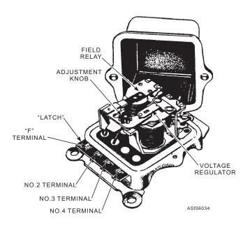
Figure 6-34.—Two-unit, vibrating-contact, ac regulator.
