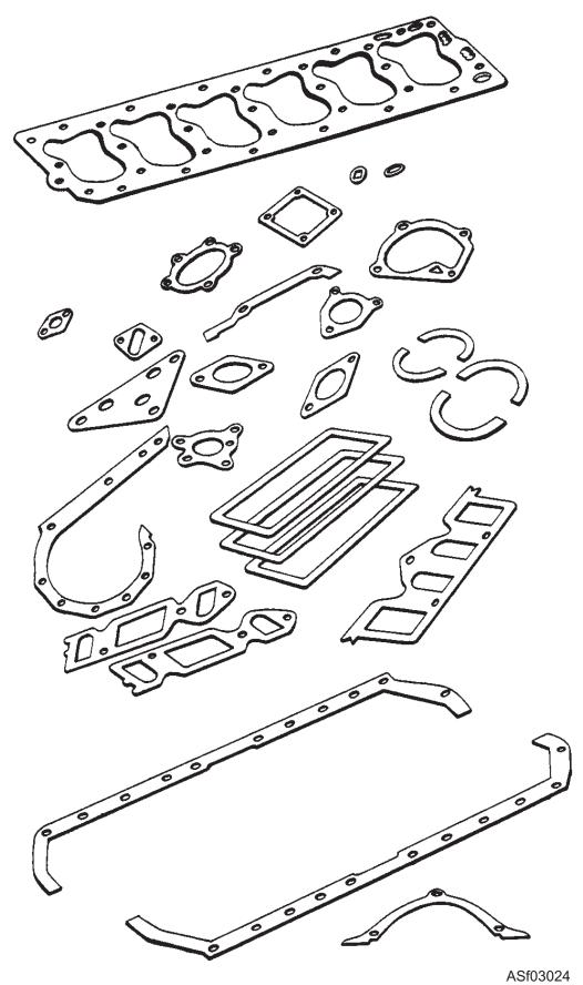
Figure 3-24.—Engine overhaul gasket kit.
