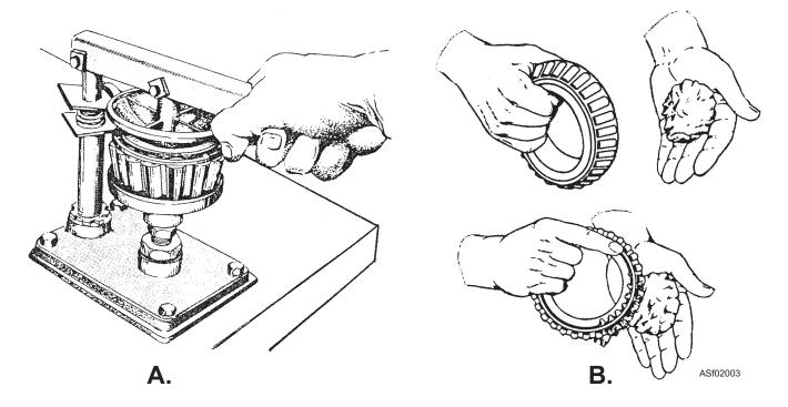
Figure 2-3.—Packing wheel bearings.
