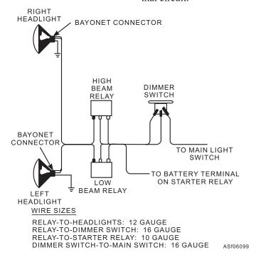
Figure 6-99.—Light relay wiring diagram.
