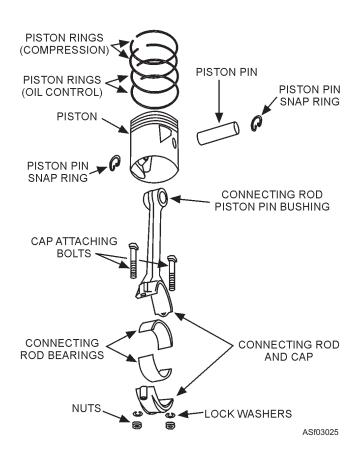
Figure 3-25.—Piston and connecting rod (exploded view).
