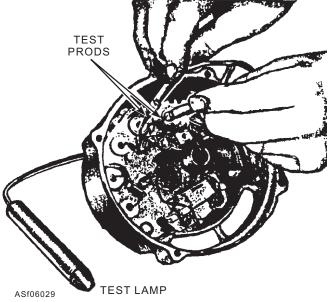
Figure 6-29.—Testing diodes with a test lamp.
