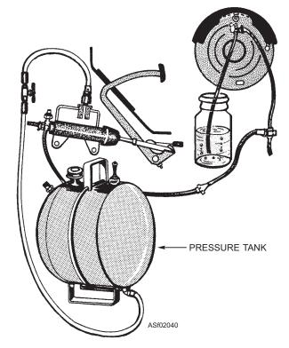
Figure 2-40.—Bleeding hydraulic system—pressure method.
