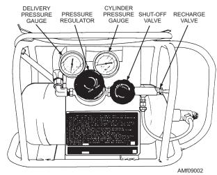
Figure 9-2.—Portable high-pressure nitrogen cylinder.
