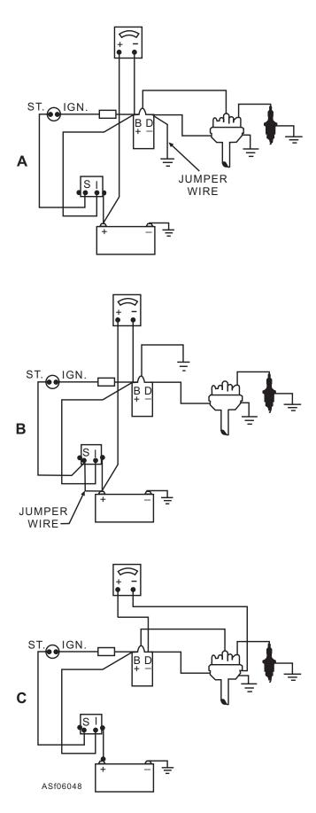
Figure 6-48.—Voltmeter connections for resistance tests of the primary circuit.
