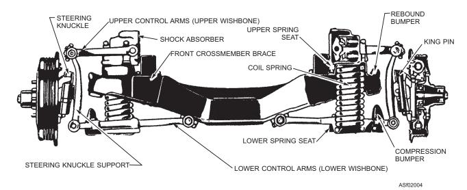
Figure 2-4.—Coil spring suspension.
