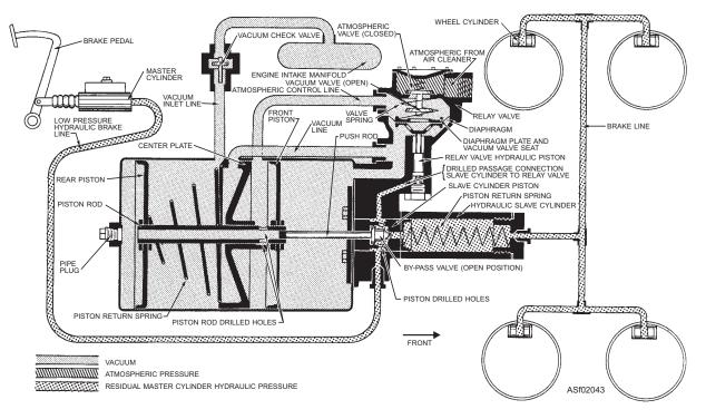
Figure 2-43.—Hydrovac operation—released position.
