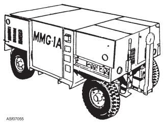
Figure 7-55.—MMG-1A mobile motor-generator set (external view).
