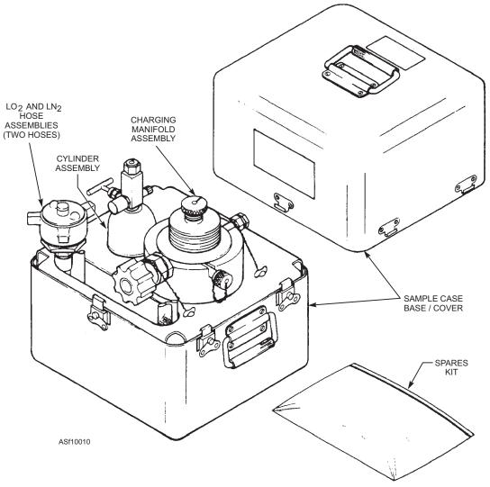
Figure 10-10.—FCS 2001 cryogenic sampler.
