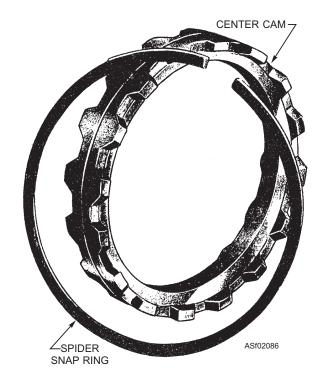
Figure 2-86.—Construction of center cam.
