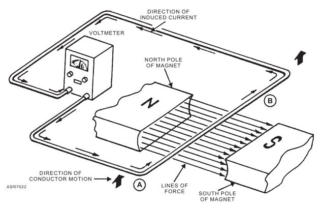
Figure 7-22.—Electromagnetic induction principles.
