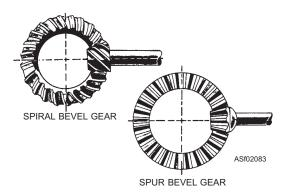
Figure 2-83.—Ring gear and pinion.
