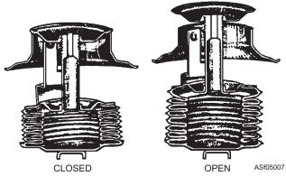
Figure 5-7.—Bellows thermostat.
