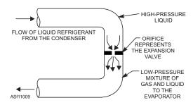
Figure 11-9.—Expansion valve principle.
