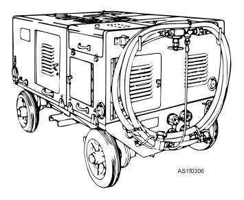
Figure 1-8.—A/M27T-5 portable hydraulic power supply.
