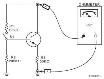
Figure 7-11.—Testing a transistor's gain with an ohmmeter.
