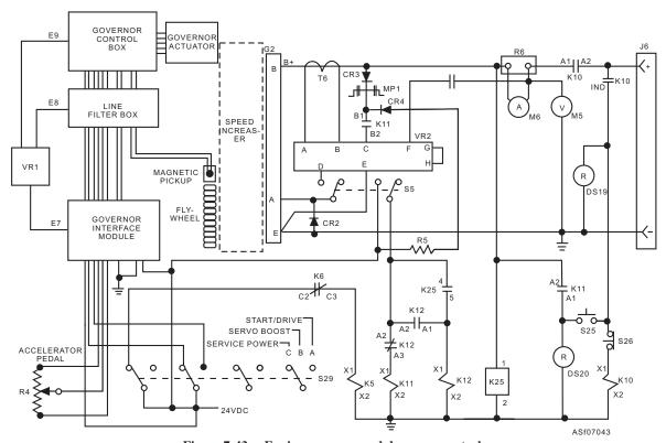
Figure 7-43.—Engine governor and dc power control.
