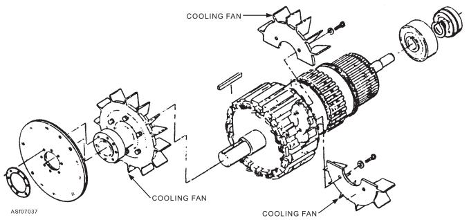
Figure 7-37.—Internal cooling fans of a typical generator.
