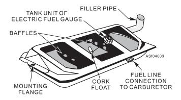
Figure 4-3.—Fuel tank with top cut away.
