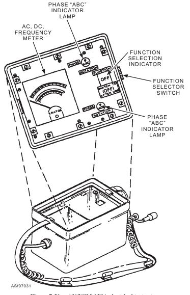
Figure 7-31.—AN/USM-128A electrical test set.
