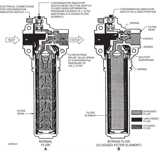
Figure 8-23.—Full flow bypass, electrical indicating hydraulic filter.
