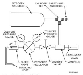
Figure 9-3.—Portable high-pressure nitrogen cylinder schematic.
