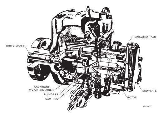
Figure 4-37.—Roosa Master fuel injection pump (Model DC).
