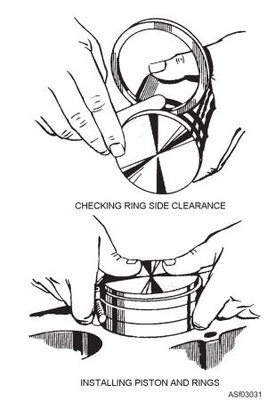
Figure 3-31.—Fitting piston ring and installing piston.
