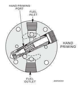
Figure 4-44.—Regulating piston during hand priming.
