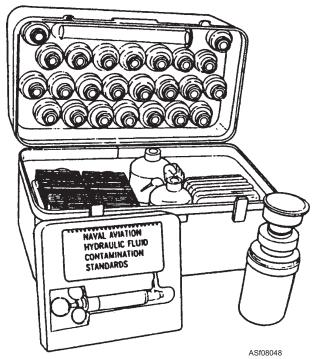
Figure 8-48.—Contamination analysis kit.
