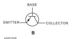
Figure 7-8.—PNP transistor—(A) PNP diagram; (B) schematic symbol.
