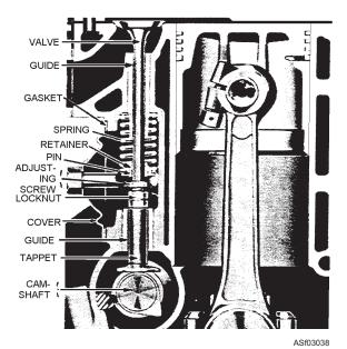
Figure 3-38.—L-head valve operating mechanism.
