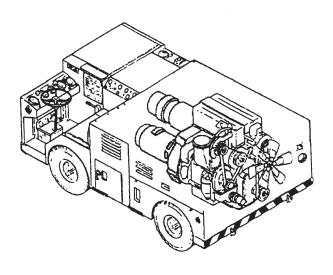
Figure 7-39.—NC-2A mobile electric power plant.
