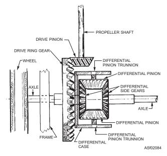
Figure 2-84.—Rear axles and differential.
