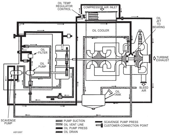
Figure 12-7.—Lubrication system.
