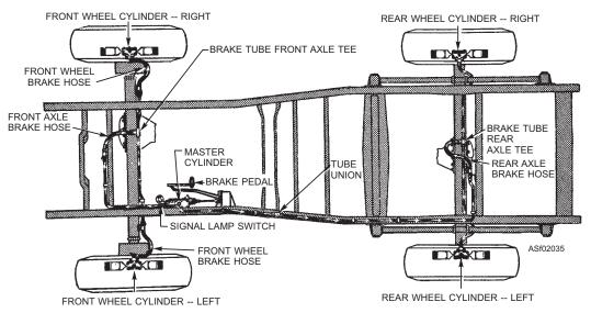
Figure 2-35.—Typical hydraulic brake system.
