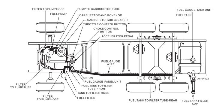
Figure 4-2.—Typical fuel system for a gasoline engine.
