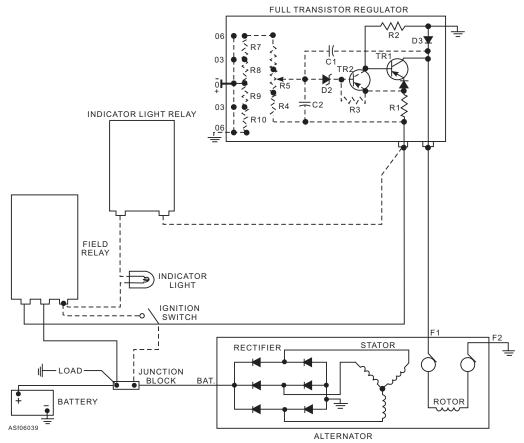
Figure 6-39.—Ac circuit using a fully transistorized regulator.
