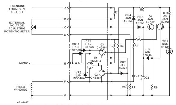
Figure 7-27.—Simplified solid-state dc voltage regulator.
