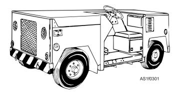
Figure 1-3.—NC-8A/A-1 mobile electric power plant.
