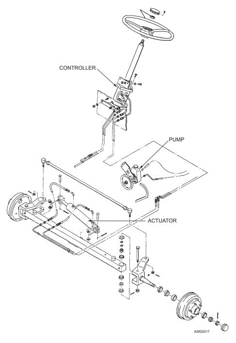
Figure 2-17.—Power steering system.
