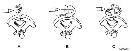
Figure 2-53.—Effects of oil jetstream on a flat surface and on a curved surface.
