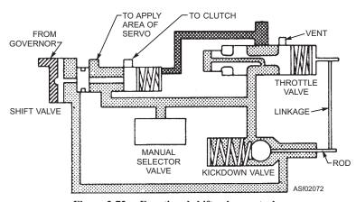
Figure 2-72.—Functional shift valve controls.
