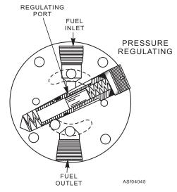
Figure 4-45.—Regulating piston in pressure regulating position.
