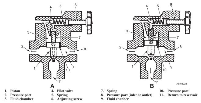
Figure 8-28.—Pilot-operated relief valve.
