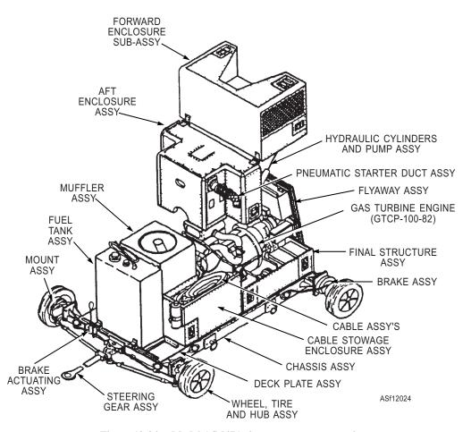
Figure 12-24.—Model A/M47A-4 compressor power unit.
