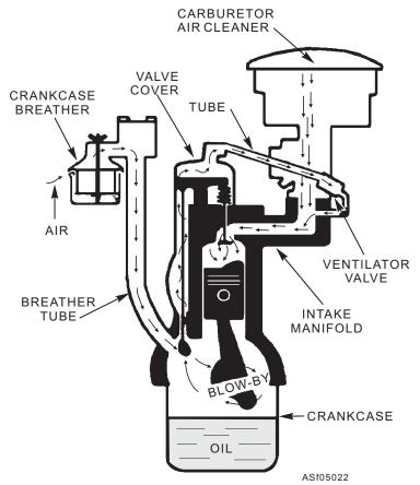
Figure 5-22.—Positive crankshaft ventilation.
