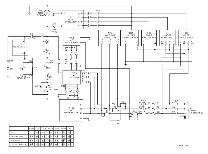
Figure 7-49.—AC power output system, simplified schematic.
