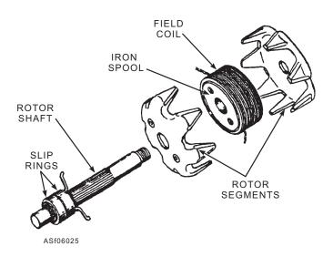
Figure 6-25.—Exploded view of an alternator rotor.
