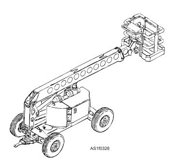
Figure 1-30.—A/S48M-2 diesel servicing platform.
