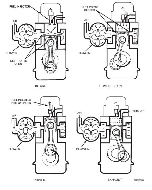
Figure 3-6.—Two-stroke cycle in a diesel engine.
