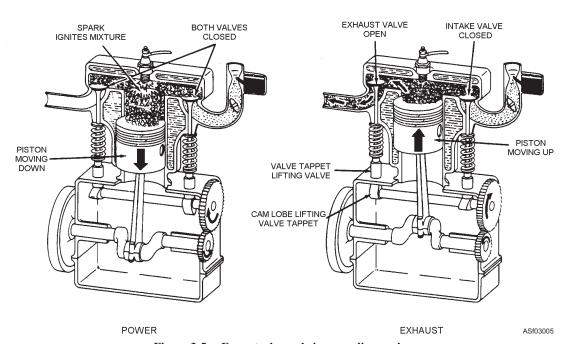
Figure 3-5.—Four-stroke cycle in a gasoline engine.
