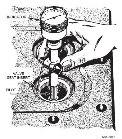
Figure 3-48.—Using a valve seat dial guage.
