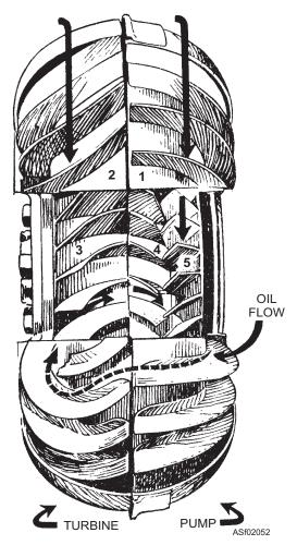
Figure 2-52.—Torque converter, multi-element.
