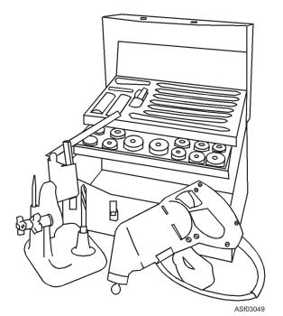
Figure 3-49.—Valve seat grinding equipment.
