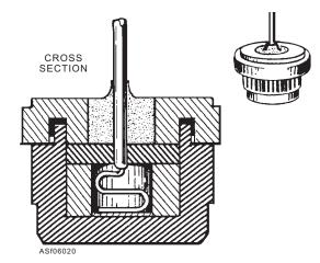
Figure 6-20.—A semiconductor (diode) rectifier.
