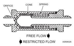
Figure 8-26.—One-way restrictor (check valve).
