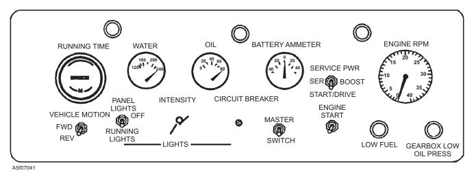
Figure 7-41.—Engine control panel.
