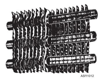
Figure 11-12.—Construction detail of an evaporator.
