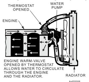
Figure 5-6.—A thermostat in operation.
