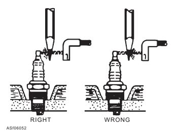
Figure 6-52.—One method of checking coil polarity.
