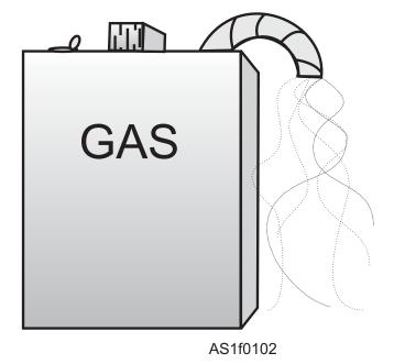
Figure 1-2.—Silhouette of gas vapors falling. Caution: Gasoline vapors are heavier than air.
