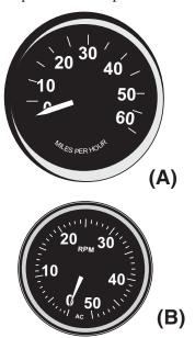
Figure 6-82.—(A) Speedometer; (B) Tachometer.
