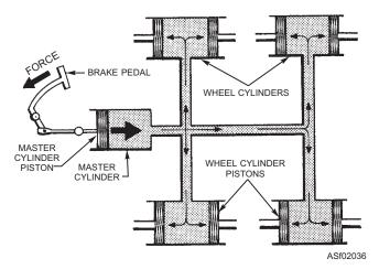
Figure 2-36.—Operation of hydraulic brake system.
