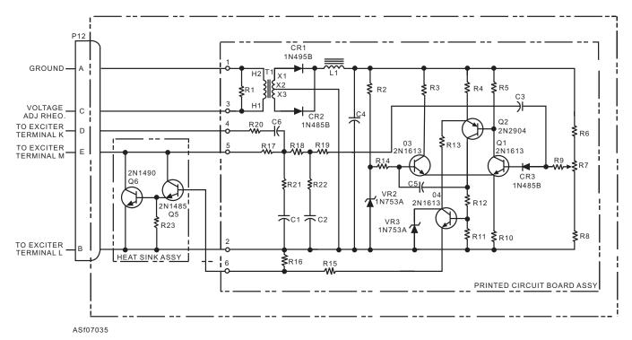
Figure 7-35.—An ac voltage regulator (VR2) simplified schematic.
