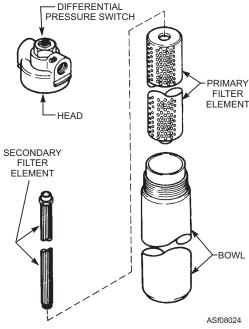
Figure 8-24.—High-pressure filter.
