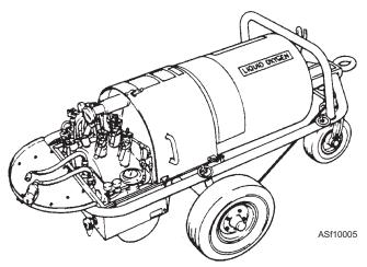
Figure 10-5.—TMU-70/M low-loss, closed-loop, liquid oxygen servicing trailer.
