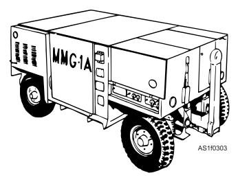
Figure 1-5.—MMG-1A mobile electric power plant.
