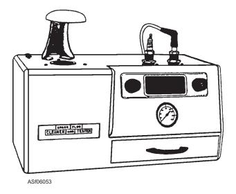
Figure 6-53.—Spark plug cleaning and testing machine.
