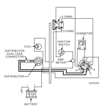
Figure 6-60.—Harness connector Nos. 4 and 5 tests.
