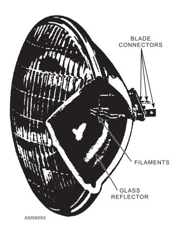
Figure 6-93.—Cutaway view of a sealed beam headlight.
