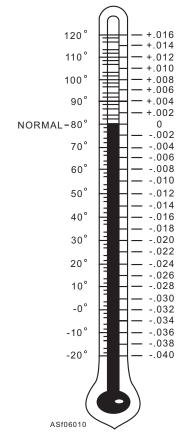
Figure 6-10.—Specific gravity temperature correction chart.
