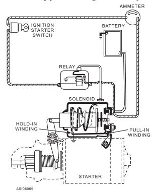
Figure 6-69.—Control system for a starter with overrunning clutch drive.
