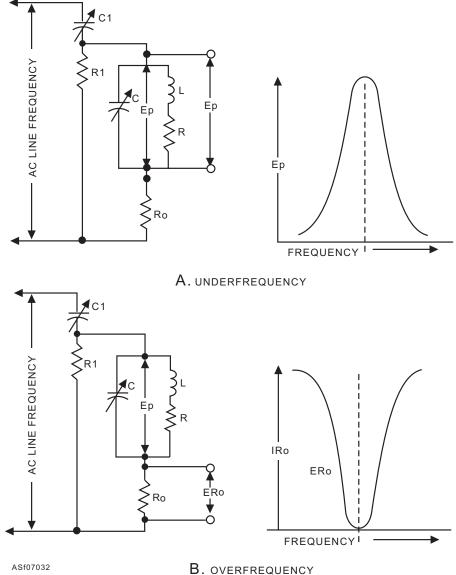
Figure 7-32.—Electrical frequency control circuits.
