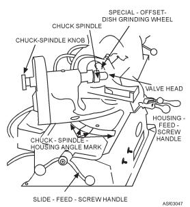
Figure 3-47.—Valve refacing machine.
