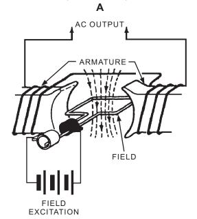
ROTATION FIELD AC GENERATOR (ALTERNATOR)
