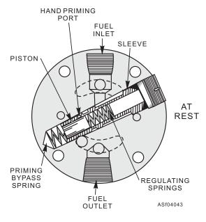
Figure 4-43.—Regulating piston at rest.
