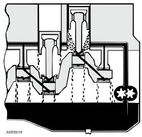
Figure 5-18.—Force-feed lubrication system.
