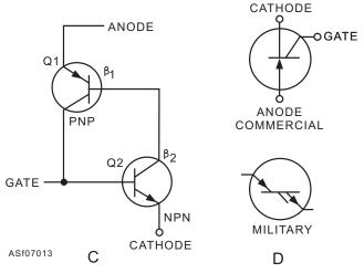
Figure 7-13.—Silicon-controlled rectifier—(A) physical PNPN structure; (B) two transistor analogy; (C) SCR internal circuitry; (D) SCR symbols.
