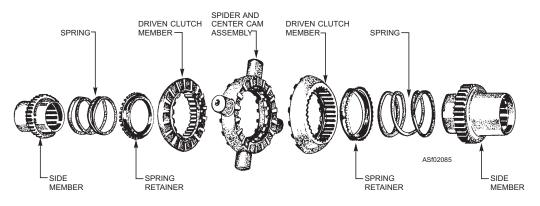
Figure 2-85.—No-spin differential disassembled.
