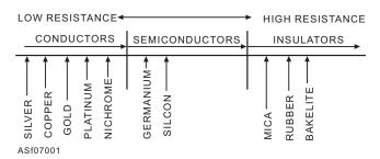
Figure 7-1.—Resistance chart of common conductors, semiconductors, and insulators.
