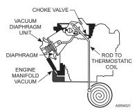
Figure 4-21.—Automatic choke with thermostatic coil mounted in manifold.
