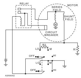
Figure 6-92.—Schematic diagram of a three-speed windshield wiper.
