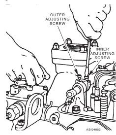
Figure 4-52.—Positioning rear injector rack control lever.
