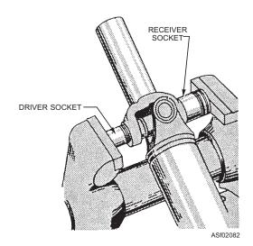
Figure 2-82.—Universal joint removal.
