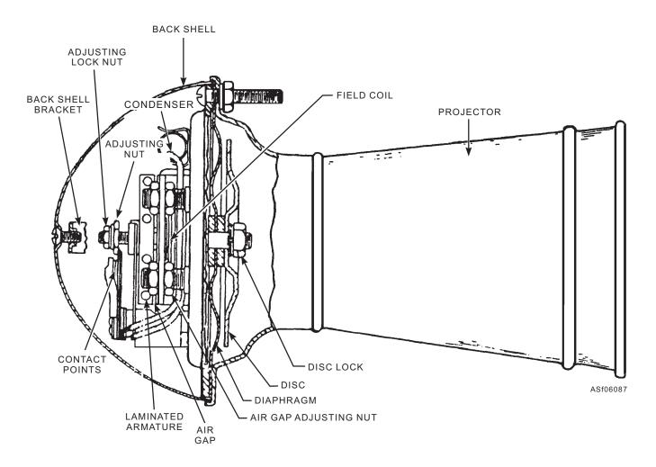
Figure 6-87.—Electrical vibrator-type horn.
