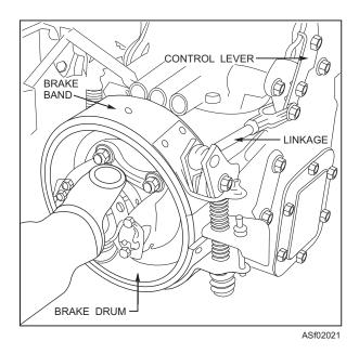
Figure 2-21.—External contracting transmission parking brake.
