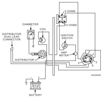
Figure 6-62.—Pickup coil ground test.
