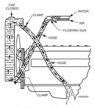
Figure 5-9.—Reverse flushing of radiator.
