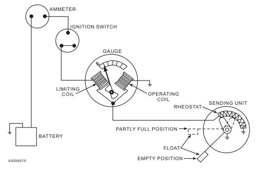
Figure 6-75.—Coil operated fuel gauge circuit.
