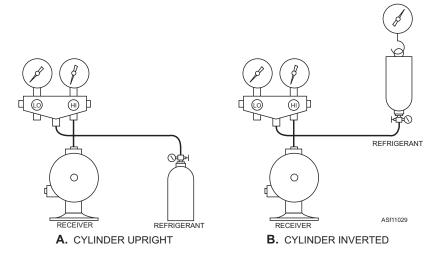
Figure 11-29.—Connections for low-side charging.
