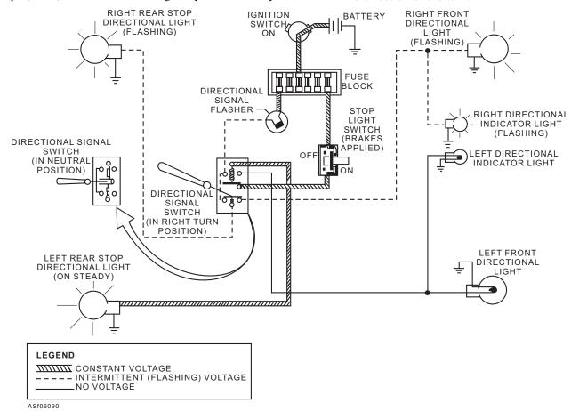
Figure 6-90.—A representative stop-directional light system.
