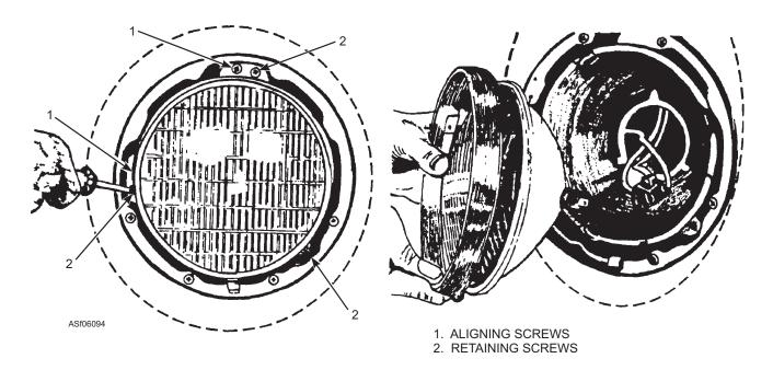
Figure 6-94.—Sealed beam headlight installation.
