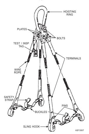
Figure 13-7.—A typical aircraft hoisting sling.
