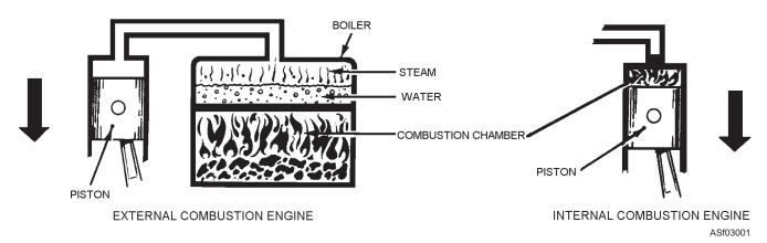
Figure 3-1.—Simple external and internal combustion engines.
