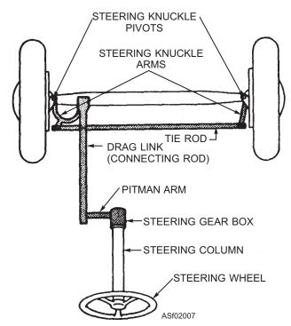
Figure 2-7.—Diagram of a steering mechanism.
