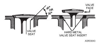
Figure 3-43.—Valve head and set angle.
