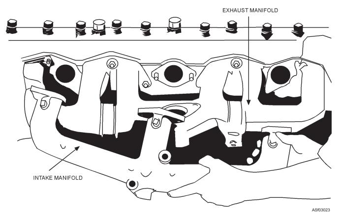
Figure 3-23.—Intake and exhaust manifolds.
