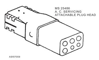
Figure 7-59.—Models of attachable head plugs.
