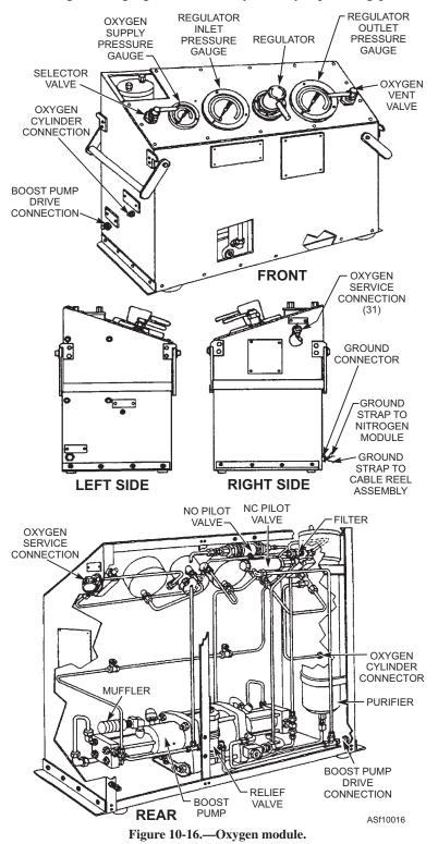
cylinder pressure with the boost pump. During aircraft oxygen servicing, the oxygen module is grounded to the nitrogen module and trailer grounding reel. The following components are contained on or within the oxygen module (refer to figure 10-16 to locate the components on the module, and to figure 10-13 to trace oxygen flow):
