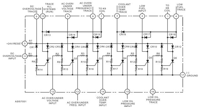
Figure 7-51.—NC-8A fault board.
