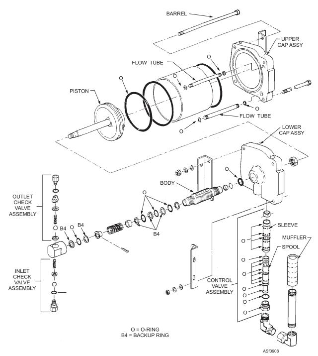
Figure 9-8.—Motor and pump assembly.
