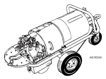
Figure 1-36.—TMU-70 liquid oxygen servicing unit.
