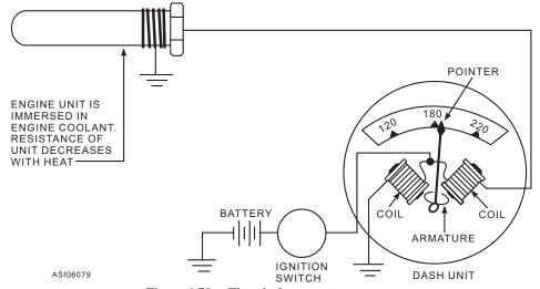
Figure 6-79.—Electrical temperature gauge.
