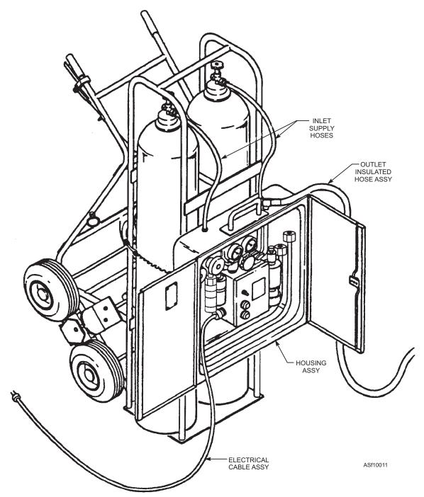
Figure 10-11.—Aircraft liquid oxygen system gas purging set.
