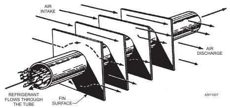
Figure 11-7.—Construction of an air-cooled condenser.
