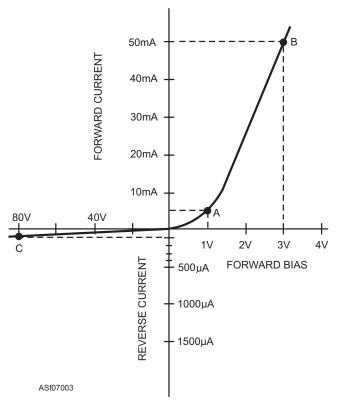
Figure 7-3.—PN junction diode characteristic curve.
