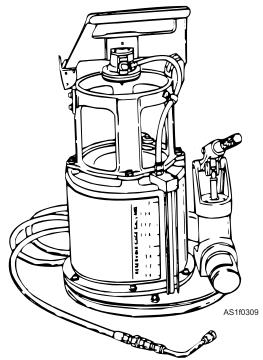
Figure 1-11.—HSU-1 hydraulic fluid servicing unit.
