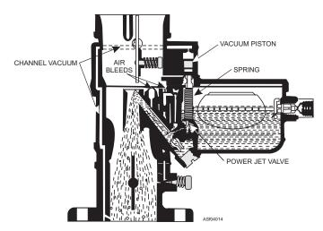
Figure 4-14.—Power jet full load circuit.
