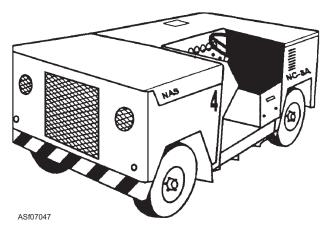
Figure 7-47.—NC-8A mobile electric power plant.
