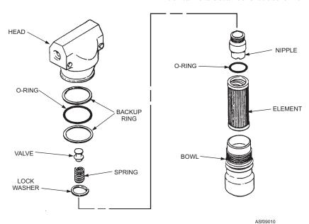
Figure 9-10.—Filter assembly.
