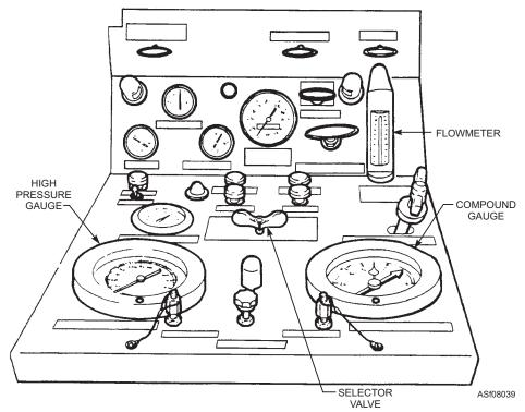
Figure 8-39.—A/M27T-5 control panel, controls, instruments, and gauges.
