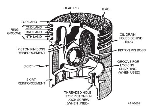
Figure 3-26.—The parts of a piston.
