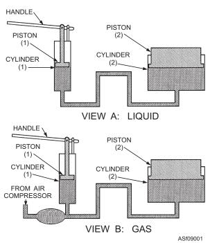
Figure 9-1.—Transmission of force by liquids and gases.
