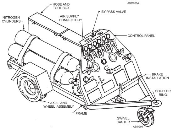
Figure 9-4.—A/M26U-4 (NAN-4) nitrogen servicing unit.
