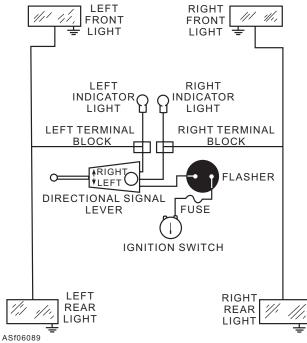
Figure 6-89.—Pictorial diagram of a directional signal system.
