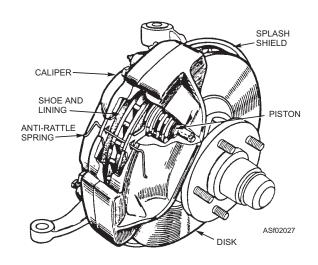
Figure 2-27.—Disc brake assembly.
