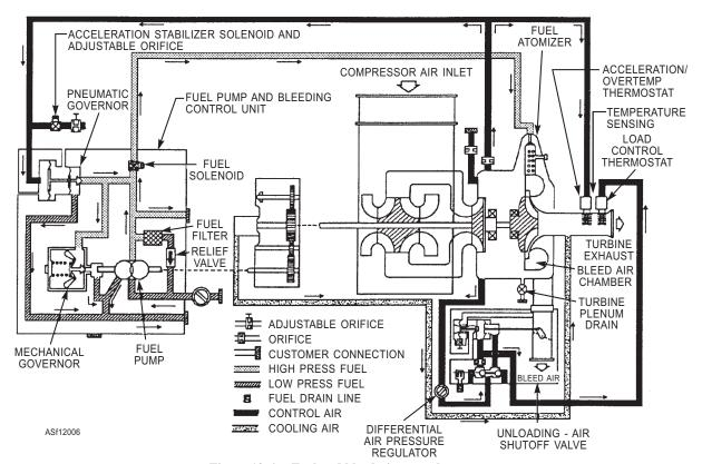
Figure 12-6.—Fuel and bleed-air control system.
