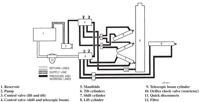
Figure 13-11.—Schematic of a typical forklift hydraulic system.
