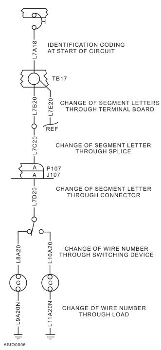
Figure 6-6.—Example of wire identification code use.
