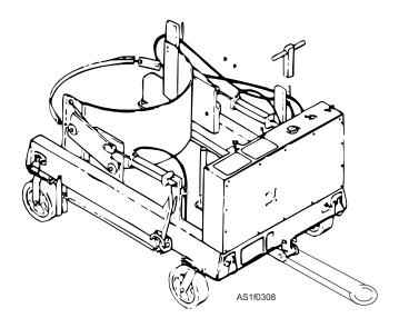
Figure 1-10.—A/M27M-10 hydraulic fluid dispensing unit.
