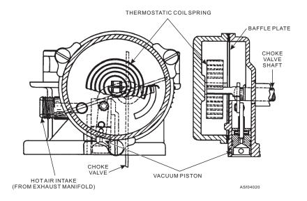
Figure 4-20.—Automatic choke.
