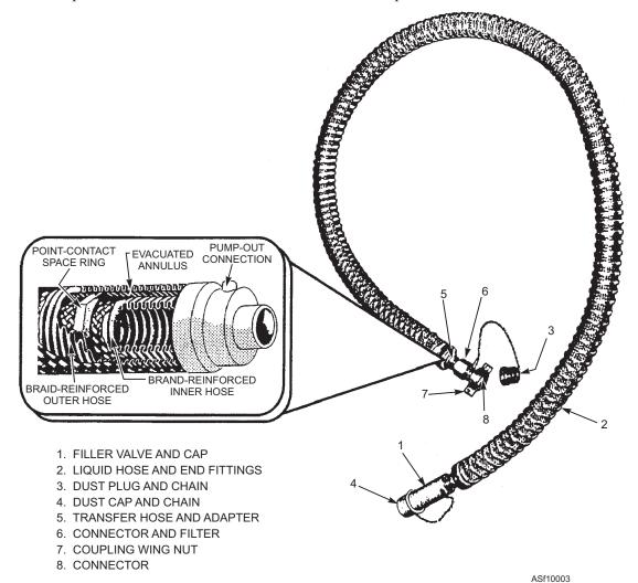
Figure 10-3.—Corrugated flexible metal hose.
