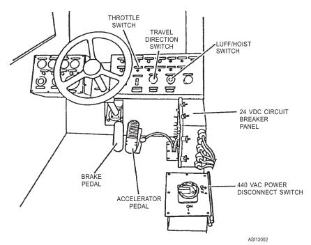
Figure 13-2.—Operator's cab.
