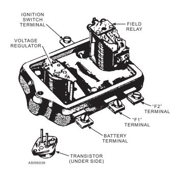
Figure 6-36.—Semitransistorized regulator.
