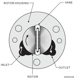
Figure 4-36.—Vanes and rotor in housing of a vane-type fuel pump.
