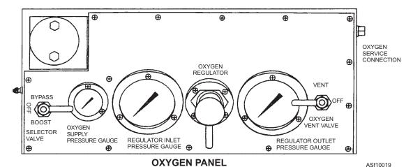
Figure 10-19.—Servicing controls and indicators.
