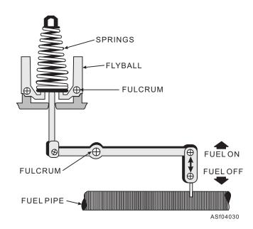
Figure 4-30.—Simple mechanical governor.
