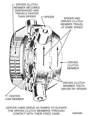
Figure 2-88.—Action of a center cam during a turn.
