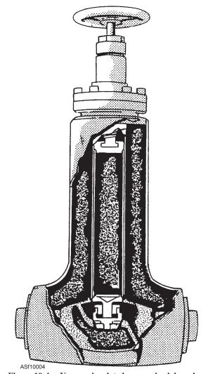
Figure 10-4.—Vacuum insulated cryogenic globe valve.
