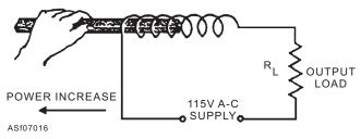
Figure 7-16.—Varying coil inductance mechanically.
