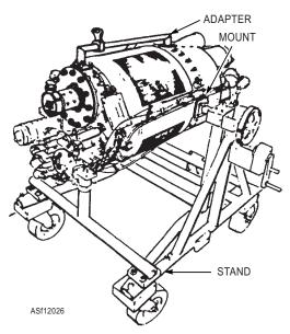
Figure 12-26.—Engine mounted on 281270-0-3 portable maintenance stand.
