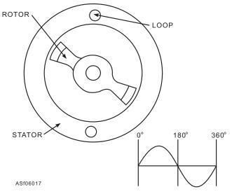
Figure 6-17.—A simple alternator.
