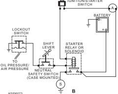
Figure 6-73.—Voltmeter connections for checking starting system circuit resistance.
