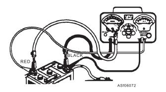
Figure 6-72.—Tester connections for a battery capacity test.
