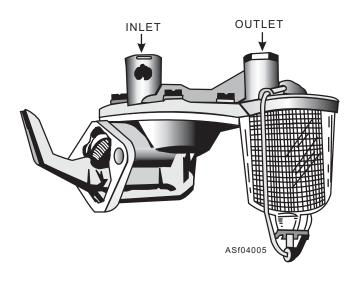
Figure 4-5.—Fuel pump with attached filter bowl.
