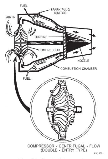
Figure 12-1.—Centrifugal-flow type engine.
