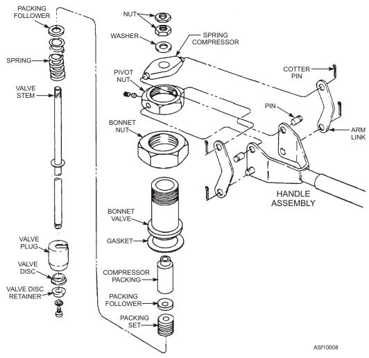
Figure 10-8.—Toggle valve assembly.
