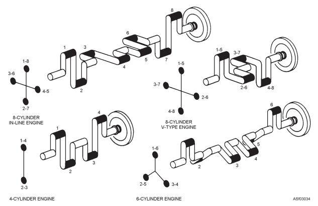
Figure 3-34.—Crankshaft and throw arrangements commonly used.
