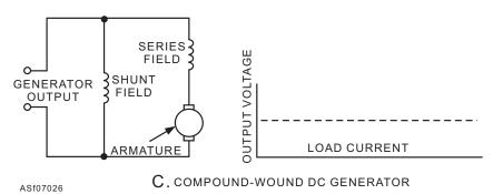
Figure 7-26.—Voltage output characteristics of the series, shunt, and compound-wound generators.
