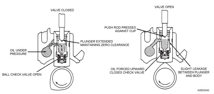
Figure 3-40.—Operation of a hydraulic valve tappet or lifter.
