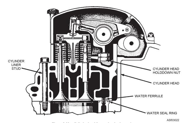
Figure 3-22.—Cylinder head for overhead valve engine.
