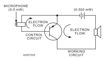
Figure 7-9.—Basic amplifying circuit.
