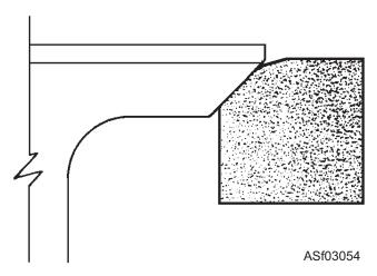
Figure 3-54.—Correct valve seat after narrowing seat.
