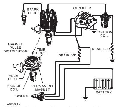
Figure 6-45.—Transistor controlled magnetic pulse battery ignition system.
