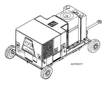
Figure 1-19.—A/M47A-4 trailer-mounted jet aircraft start unit.
