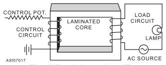
Figure 7-17.—A basic magnetic amplifier.
