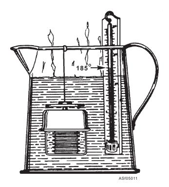
Figure 5-11.—Testing a thermometer.
