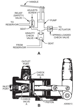
Figure 8-13.—Single-action hydraulic hand pump.
