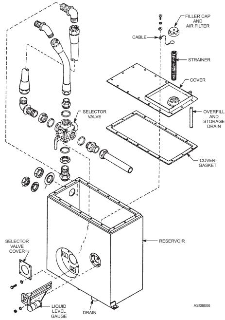
Figure 8-6.—Hydraulic Reservoir Assembly A/M27T-5.
