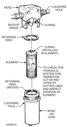
Figure 8-19.—T-type micronic filter assembly.
