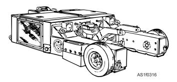
Figure 1-18.—A/S32A-32 aircraft towing tractor.
