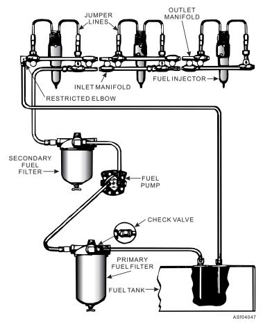
Figure 4-47.—Diagram of typical General Motors diesel fuel system.
