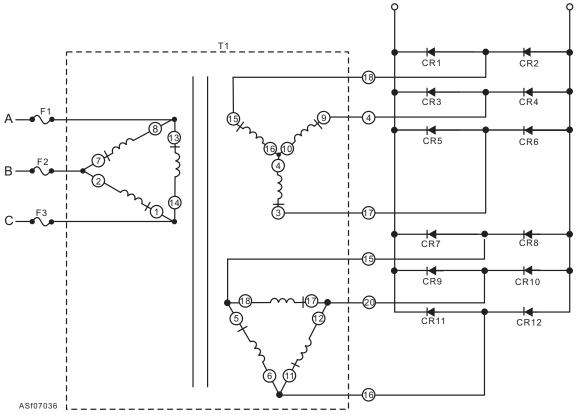
Figure 7-36.—A dc power supply circuit.
