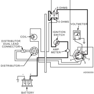
Figure 6-59.—Harness connector No. 3 test.
