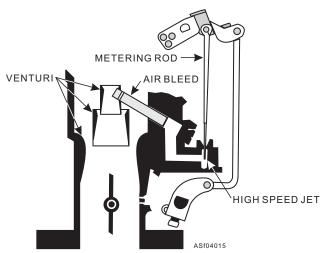
Figure 4-15.—Metering rod full load circuit.
