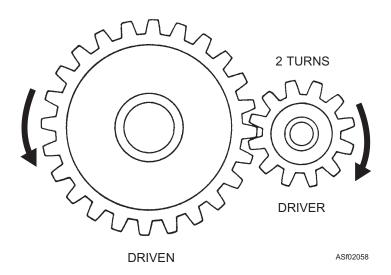
Figure 2-58.—Gear speed ratio.
