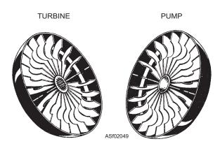
Figure 2-49.—Fluid coupling pump and turbine.
