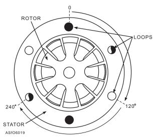
Figure 6-19.—A three-phase alternator.
