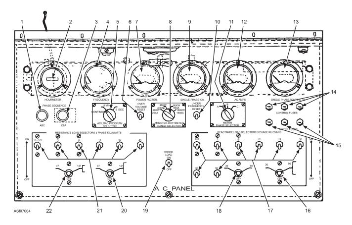
Figure 7-64.—AC control panel.
