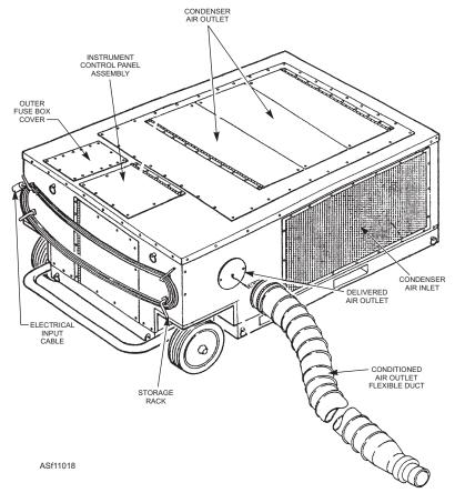
$Figure~11\text{-}18. \color{red} - A/M32C\text{-}21~trailer-mounted~air-conditioning~unit,~electric-powered.}$
