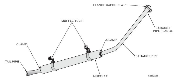
Figure 4-25.—Exhaust pipe, muffler, and tail pipe.
