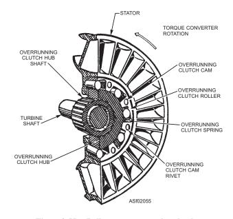
Figure 2-55.—Roller-type overrunning clutch.
