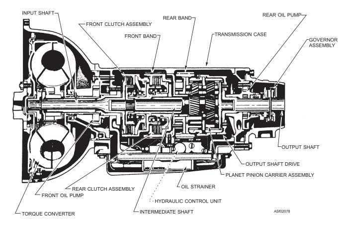
Figure 2-78.—Typical automatic transmission.
