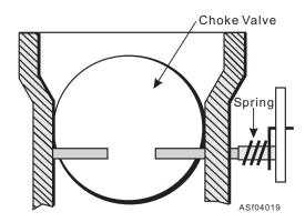
Figure 4-19.—Off-center choke valve.
