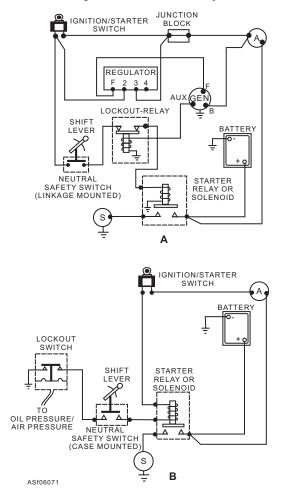
Figure 6-71.—Starter safety control combinations.
