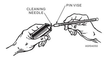
Figure 4-50.—Cleaning injector spray nozzle holes.
