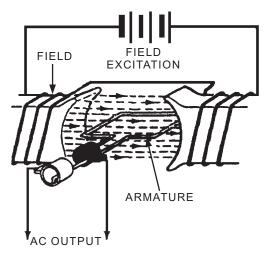
ROTATION ARMATURE AC GENERATOR (ALTERNATOR)
